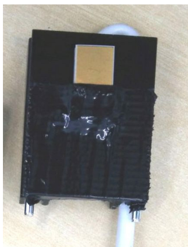
(a) 1x1cm Peltier device (gold) attached to heat-sink (black)
