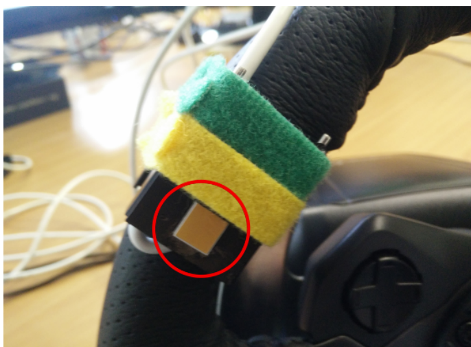
(b) Peltier device mounted on steering wheel with Velcro cable binders
