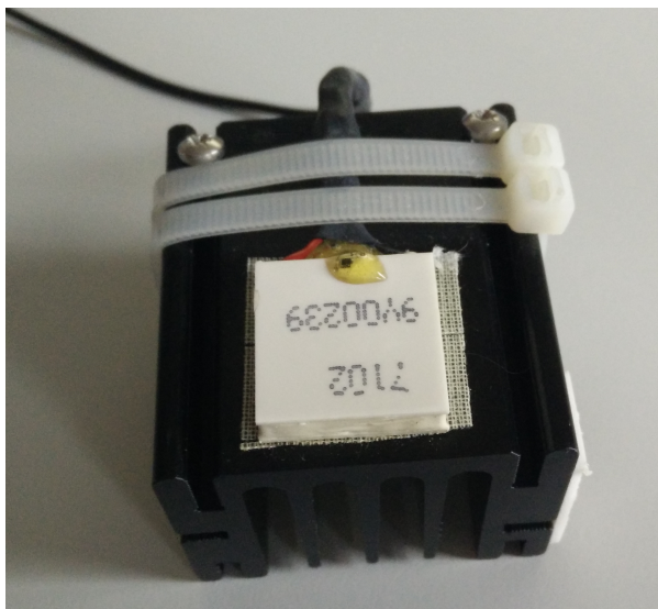
Figure 2.3: Peltier device (white) attached to heat-sink (black).
