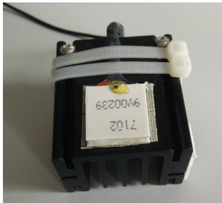
(a) Peltier element with heat-sink
