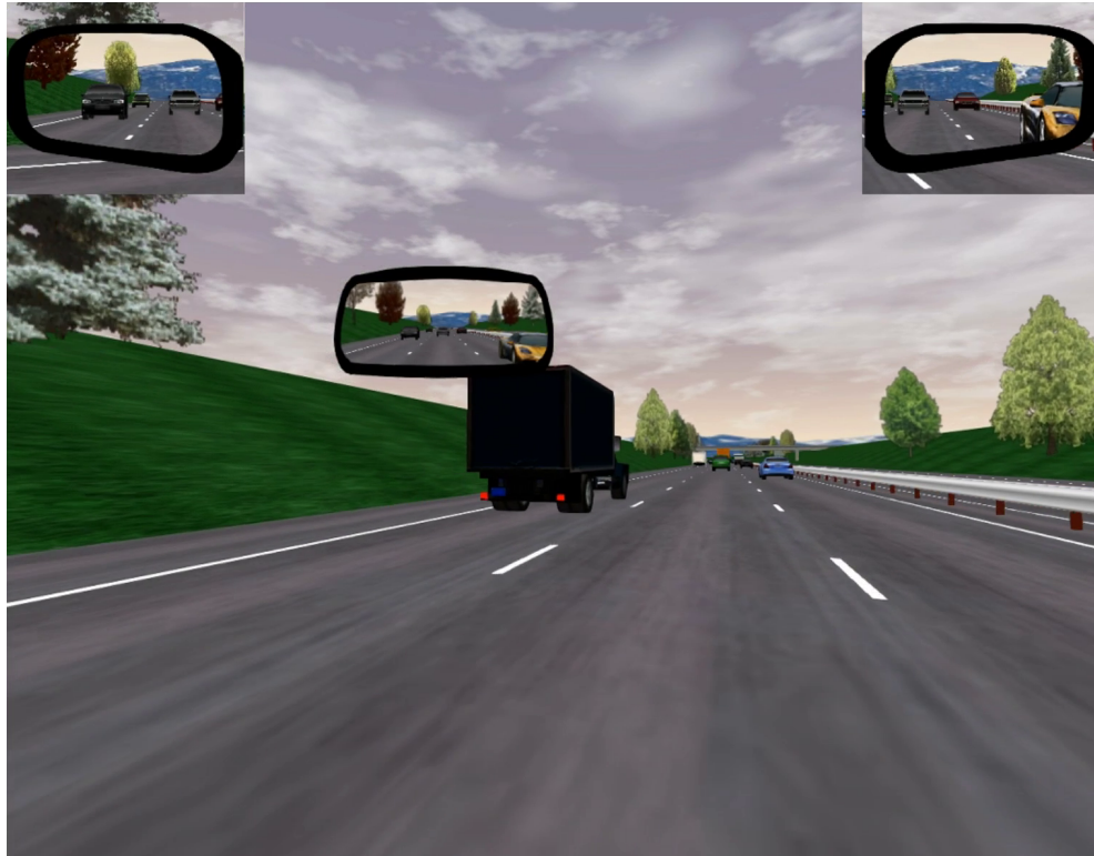
Figure 5.21: Experiment 7: Driving simulator environment as captured in the video log. The side mirror content was presented to drivers on screens at the side of the driving cabin.
