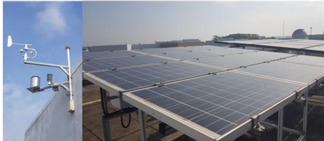
Figure 6.1 Left: Meteorological Measuring Instruments for rainfall, wind direction, and wind speed. Right: Rooftop solar panel testbed.
