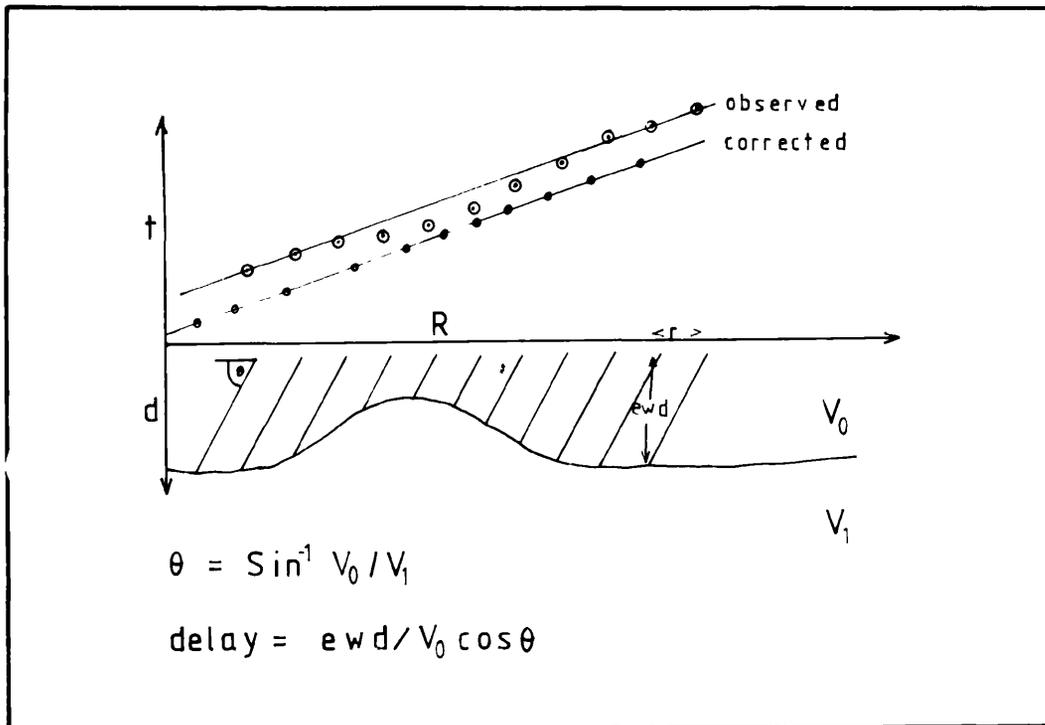
Fig 3.33 Water layer correction
