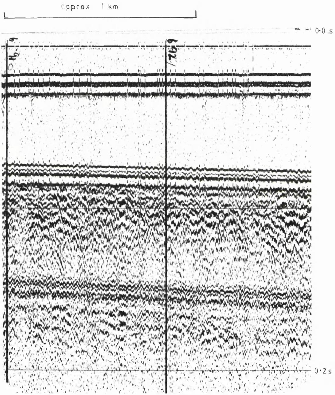
Fig 3.62 Sparker profile of probable boulder clay
