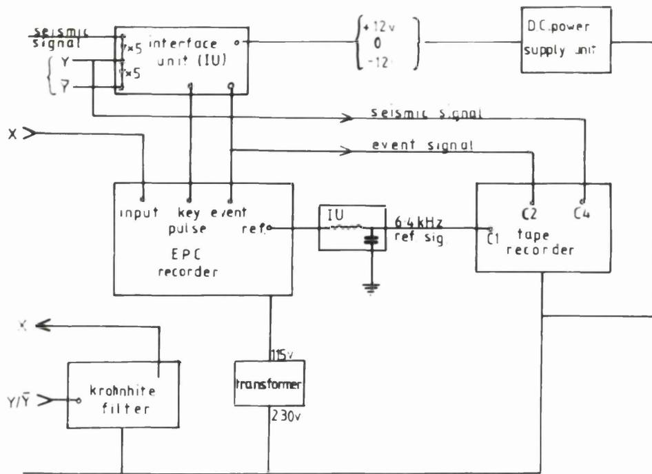
Fig 2-2a Schematic circuit diagram for recording seismic data.
