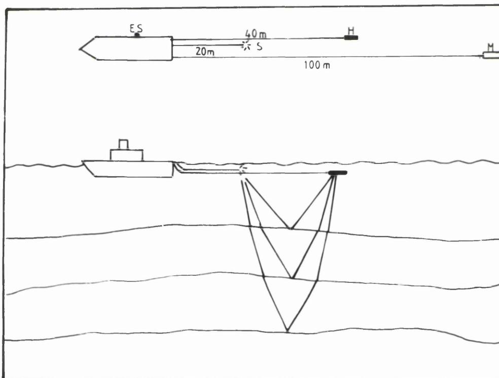
H-hydrophone S-sparker M-magnetometer ES-echo sounder
