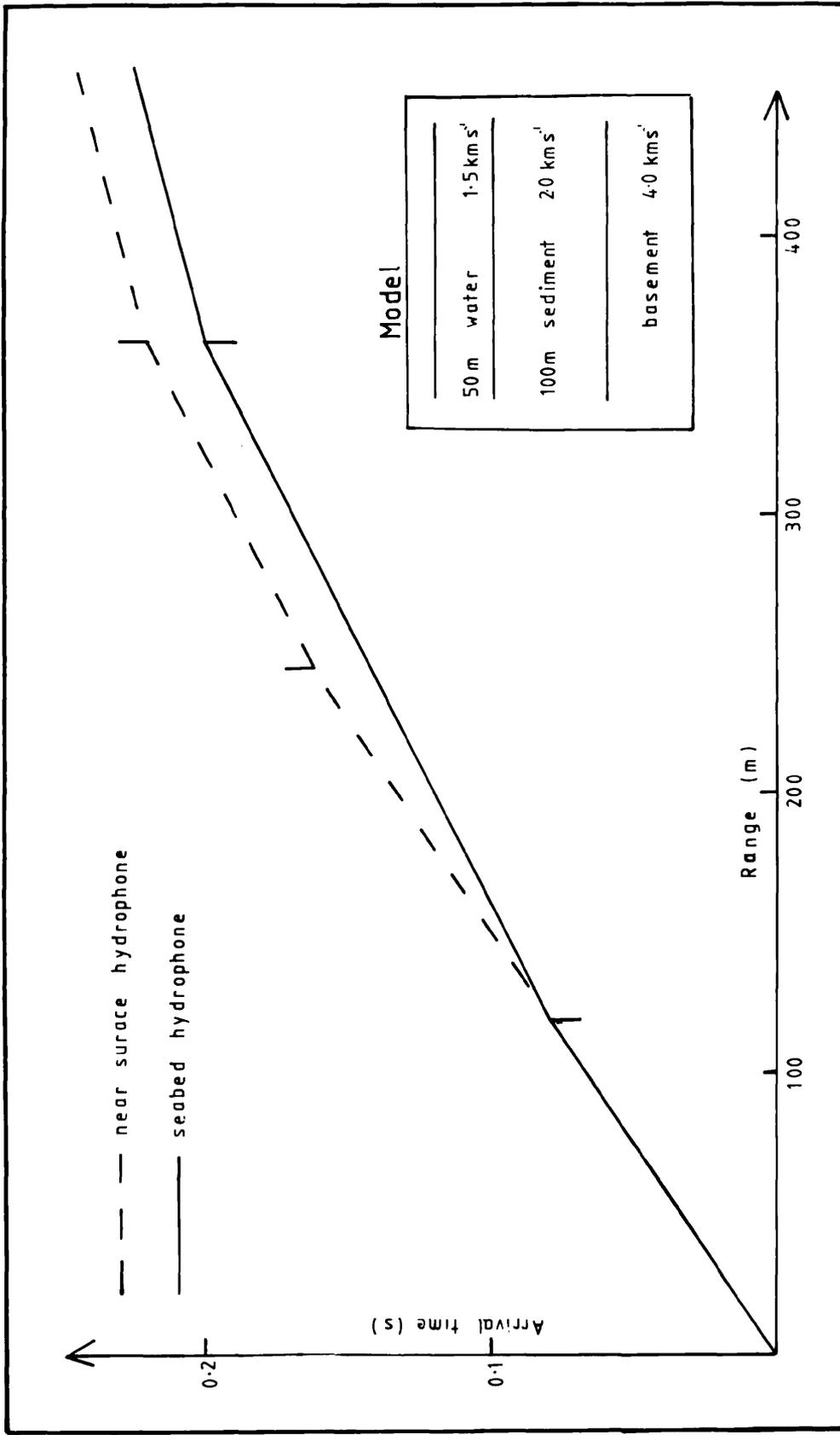
Fig 2.4 Comparison between near surface and seabed hydrophones
