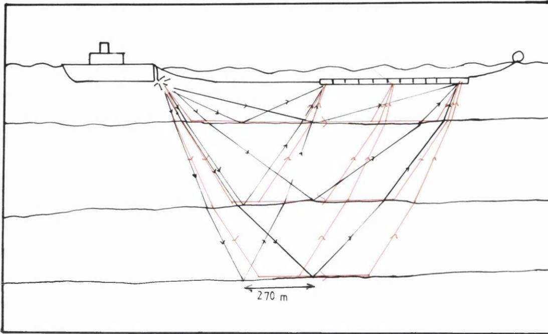
Fig 2·6 Seismic array profiling
