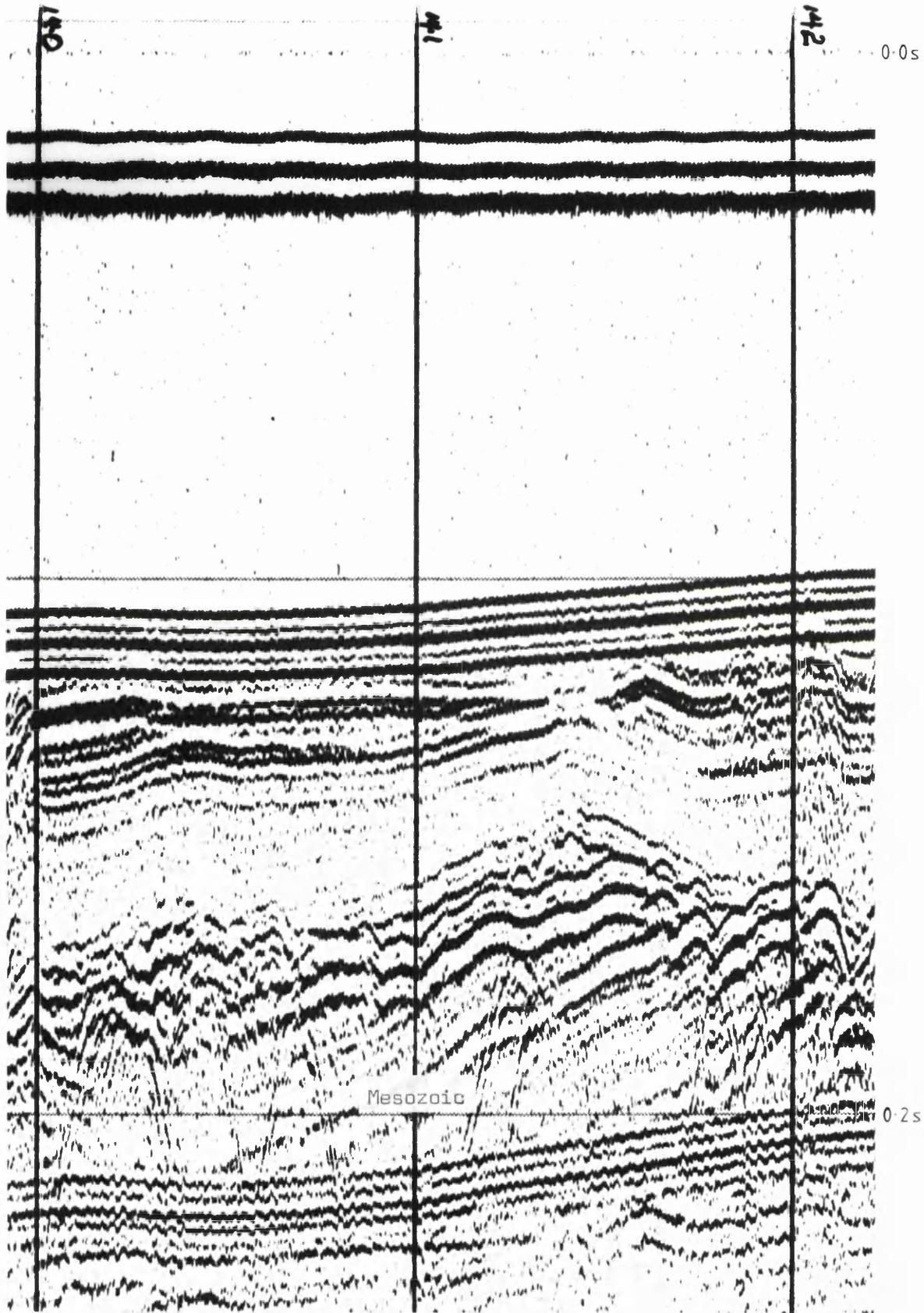
Fig 5.7 Sparker profile of Mesozoic strata
