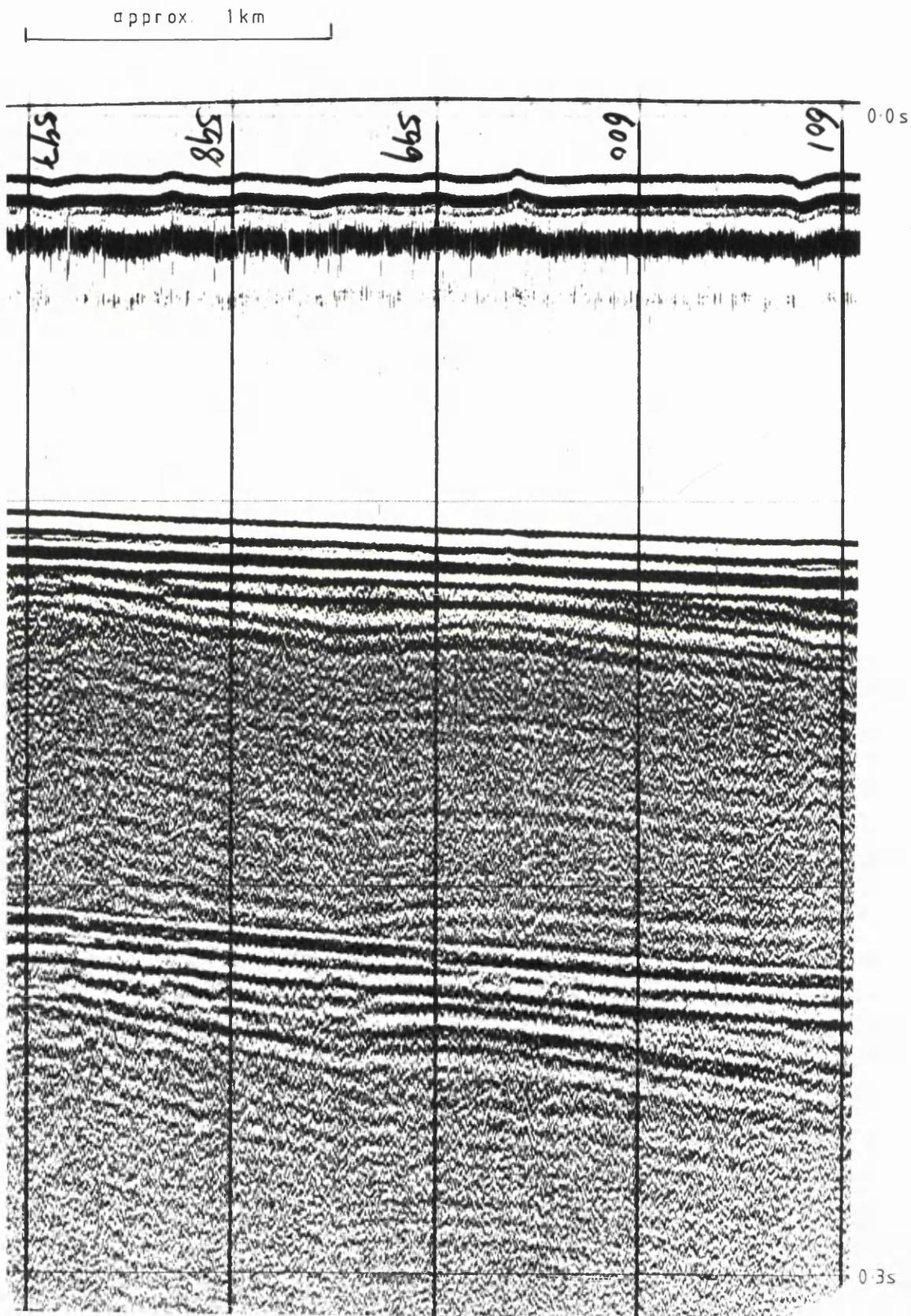
Fig 3.5 Sparker profile of recent sediment
