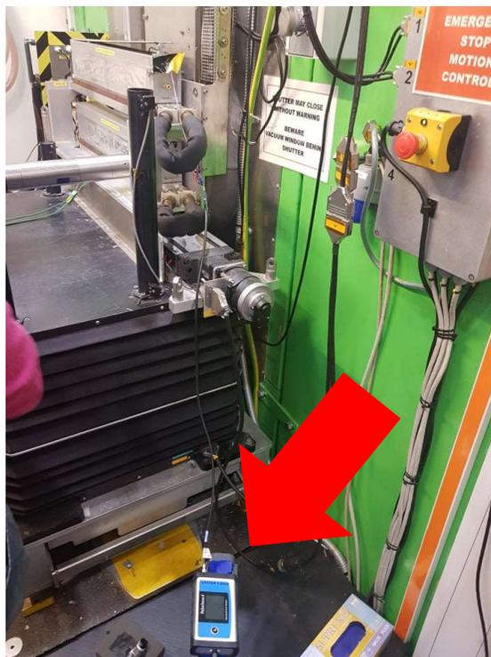
**Figure 3.40.** Connection to PalmSense Potentiostat to cell in the beamline (covered by protective foil). Potentiostat is highlighted by red arrow.
