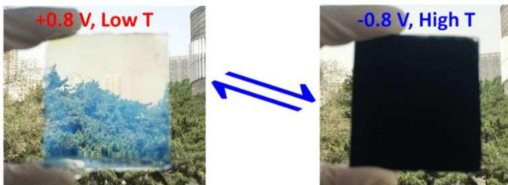
**Figure 1.3.** Photographs of the AuPR/WO<sub>3</sub> film on fluorine-doped Sn oxide (FTO) at the bleached state and the coloured state. Reproduced from Xu *et al.*<sup>58</sup>
