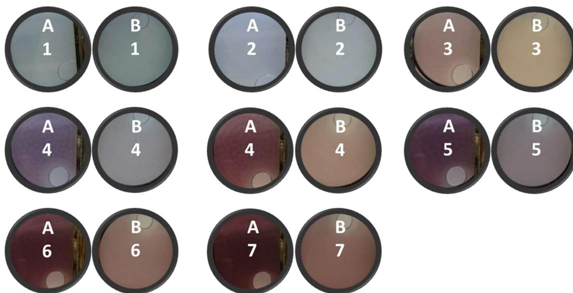
**Figure A.3.23.** Images of FTO windows filled with **NDI-I** at 10 mg/mL exposed to natural daylight without (A) and with (B) UV filter protective film. A1 and B1 represent the solution at the start of the experiments and images following were taken every 30 minutes of exposure to natural light, starting with A1 and B2 until A7 and B7 (images after 3 hours 30 minutes).
