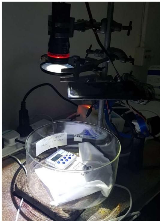
**Figure 3.37.** Photograph showing the set-up in which cycling test are run.
