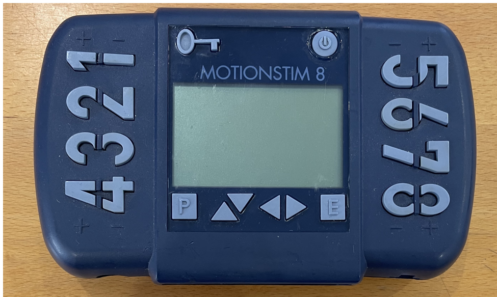
Figure 3.4: The functional electrical stimulator (FES) used to generate the electrotactile cues.
