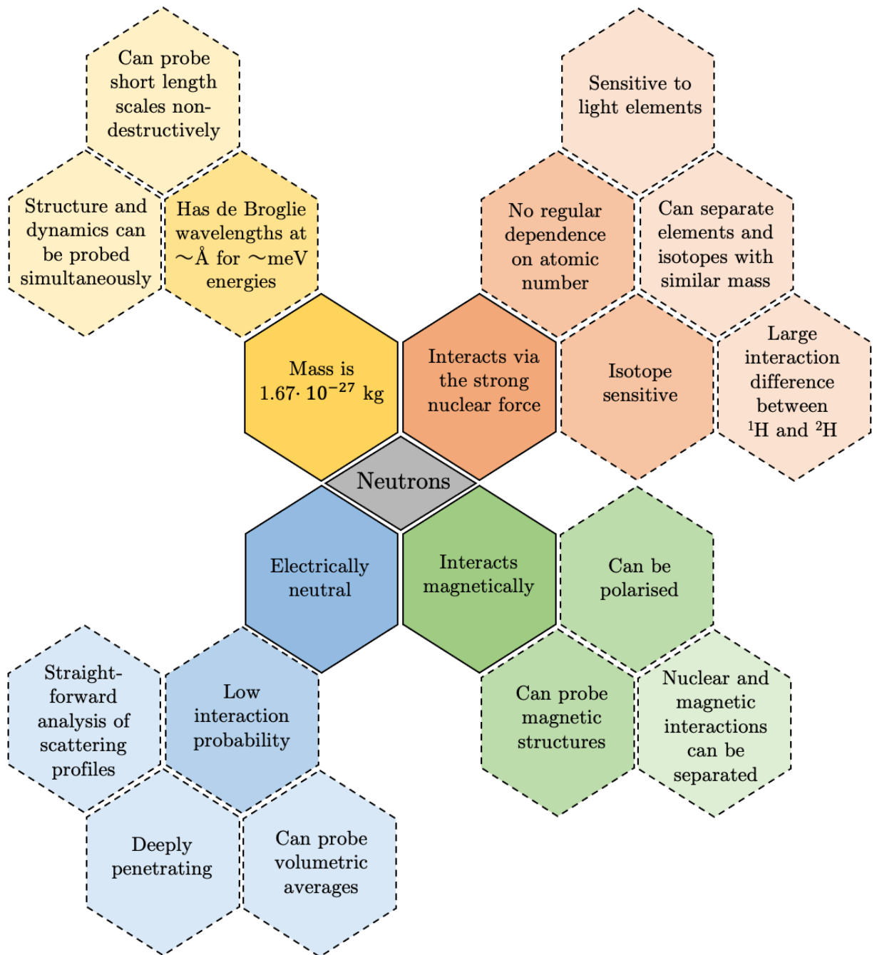
Figure 1.1: An overview of relevant neutron properties. In the centre, four neutron attributes are shown (solid hexagons). These are neutron mass, strong interaction, electrical neutrality and magnetic interaction. From these attributes, their useful consequences (dashed hexagons) are mapped out.
