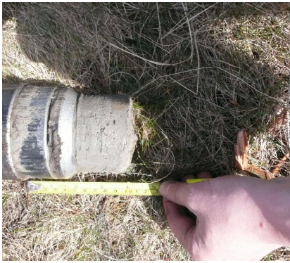
Figure A- 1: Sandy base of MR8 core (5cm) that got damaged from the rest of the core
