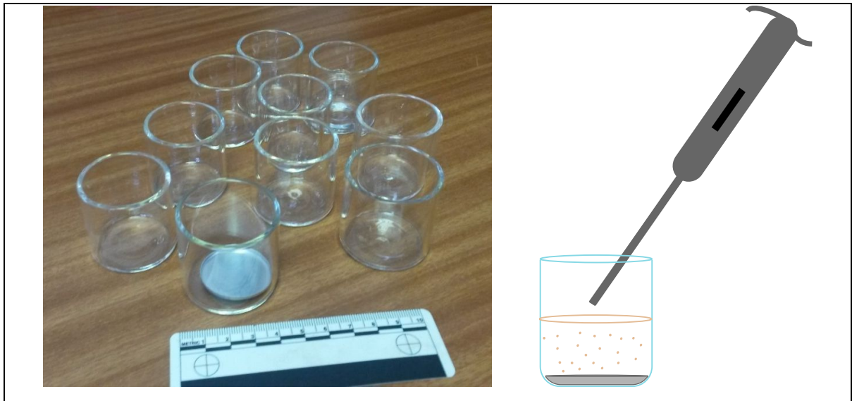
Figure 7-21: Custom made glass jars (left) by Robert McLeod and Calum Prentice in the SUERC glassblowing workshop for making these used to receive pipetted < 30 \mu\text{m} grain in acetone and dispense on 3cm aluminium planchettes.
