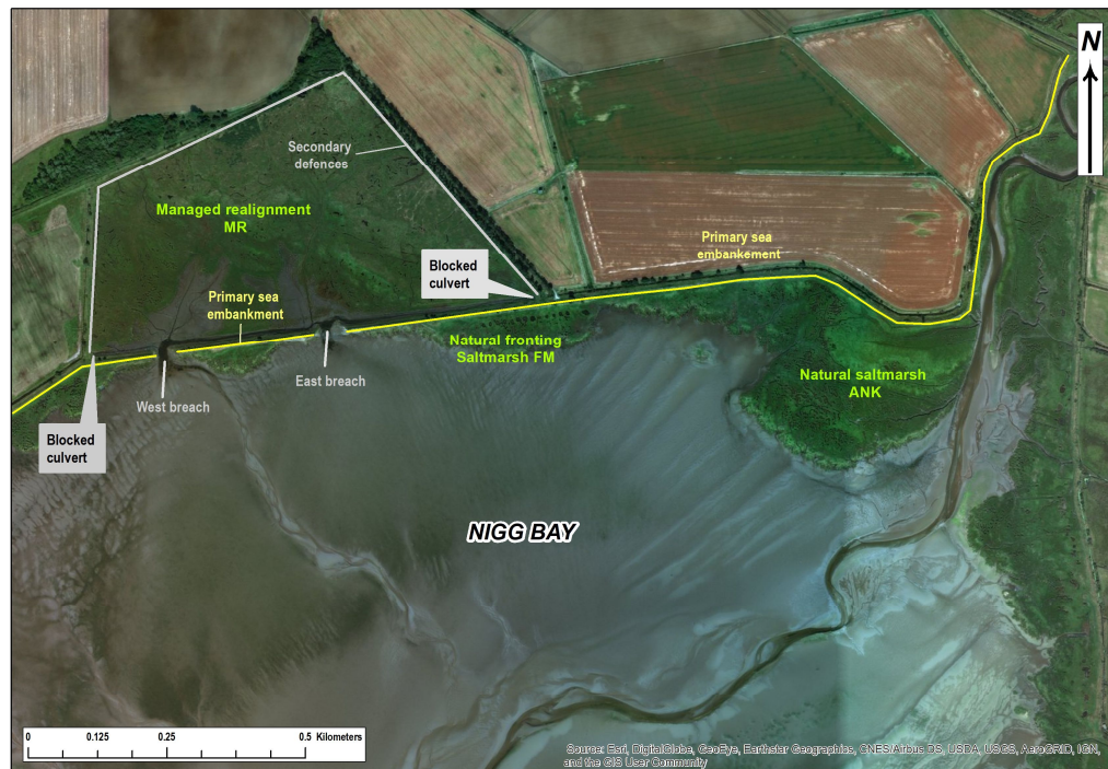
Figure 3-7: Nigg Bay post-realignment showing secondary defences (grey), blocked culverts (grey) constructed in advances of the two breaches (east and west in grey) through primary sea embankment (1950s in yellow) with the location of three research study sites.
