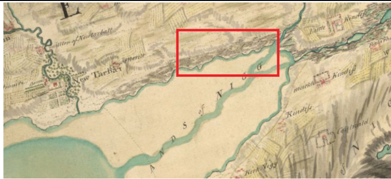
NB: Roy's map cartographic style uses Yellow for cultivated ground; Dark green for woodland and blue-green for water parallel with hatching for tilled land and stipple for sands or shoals) (from NLS, https://maps.nls.uk/roy/style.html )
