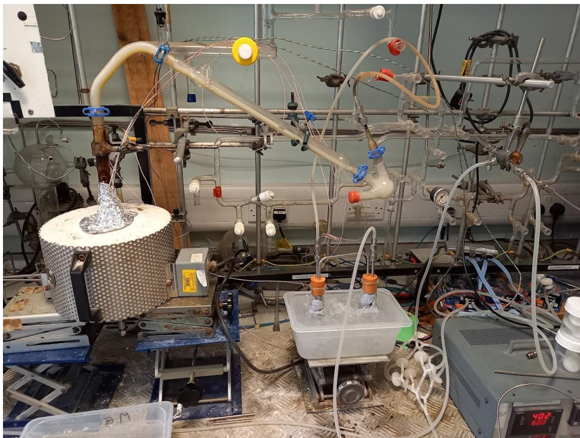
Figure 6-2: Heated reactor and tar removal components of the experimental setup. From left to right the heater and reactor, the straight condenser tube, the ice bath and condenser flasks, PTFE filters, and temperature controller.
