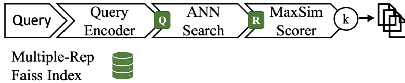
Figure 2.9: Conceptual Architecture of Multiple Representation Dense Retrieval using PyTerrier.
