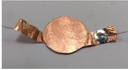
Figure 6-6 Conductive copper tape placed on both faces of a PZT disk with copper wires soldered in opposite directions.
