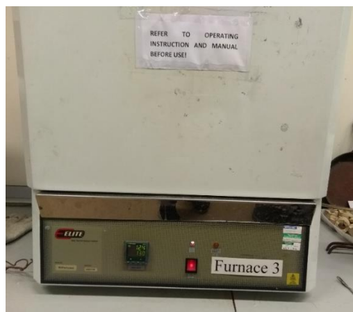
Figure 3-21 Elite Chamber Furnace used for HP sample sintering.
