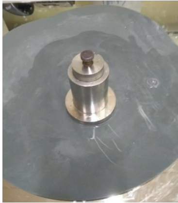
Figure 5-3 Sample holder on top of wet silicon carbide lapping paper.
