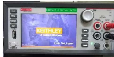
Figure 6-11 DMM7510 Keithley multimeter used to collect the I-V data from the coupled PZT samples.
