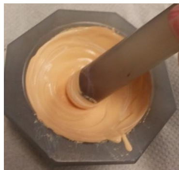
Figure 3-7 Wet hand grinding of PZT done with previous samples.
