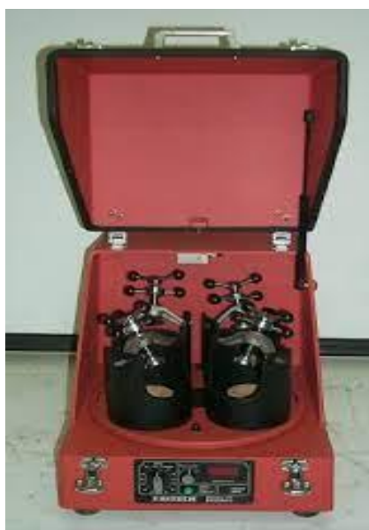
Figure 3-6 Fritsch® pulverisette 5 planetary ball mill and inner container holder with counterweight.
