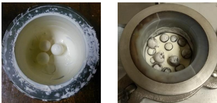
Figure 3-16 Wet LP (left) and HP (right) PZT mix after second ball milling.
