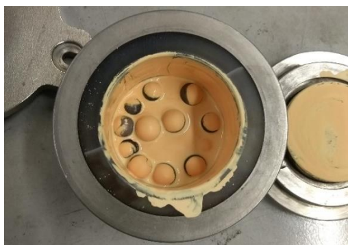
Figure 3-4 Ball mill agate container with HP PZT wet mix and twenty 1 cm agate balls.
