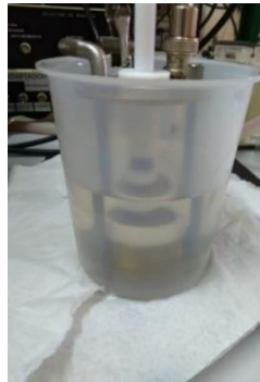
Figure 5-12 Front view of the sample holder submerged in dielectric fluid (FC40).
