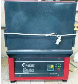
Figure 3-12 Vecstar chamber muffle furnace with Eurotherm 2416 controller.
