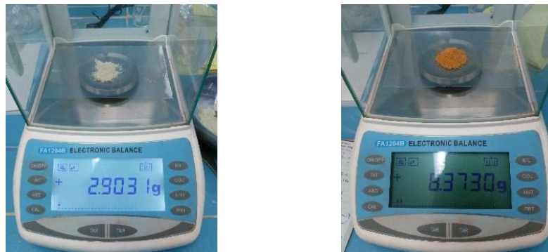
Figure 3-2 Analytical scale FA1204B weighing low purity \text{ZrO}_2 (left) and \text{PbO} (right).
