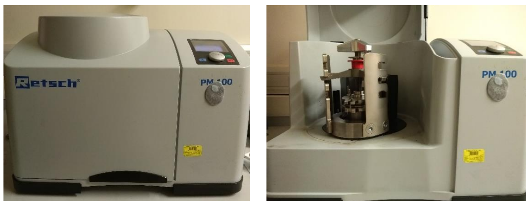
Figure 3-5 Retsch® planetary ball mill PM 100 and inner container holder with counterweight.
