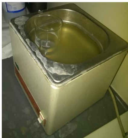
Figure 5-6 PZT pellet being cleaned with ethanol inside an ultrasonic bath.
