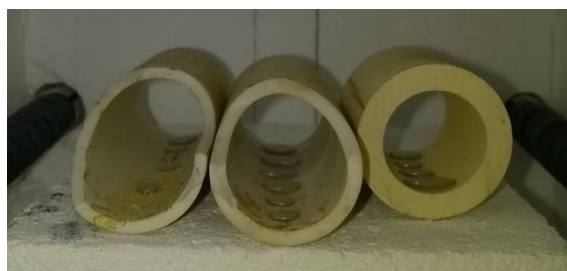
Figure 5-9 Alumina crucibles holding the silver-coated small PZT sample pieces inside the Energon furnace before the paint is cured at 600°C for 1h.
