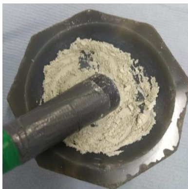
Figure 3-20 Agate pestle and mortar used to incorporate PVA binder to calcined PZT powders.
