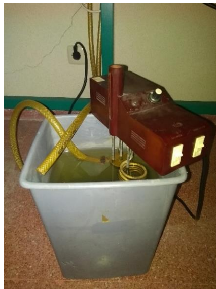
Figure 5-21 Cooling mechanism employed during the poling of the PZT samples.
