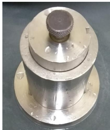
Figure 5-2 Steel sample holder used for lapping the PZT disks from each composition.
