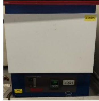
Figure 3-13 Lenton Chamber Furnace with Eurotherm 3216 controller.
