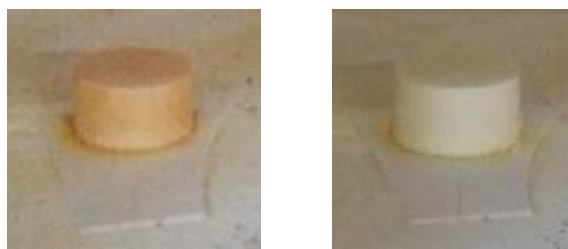
Figure 3-14 LP 0.47 PZT compressed pellet before (left) and after (right) calcination at 800°C.
