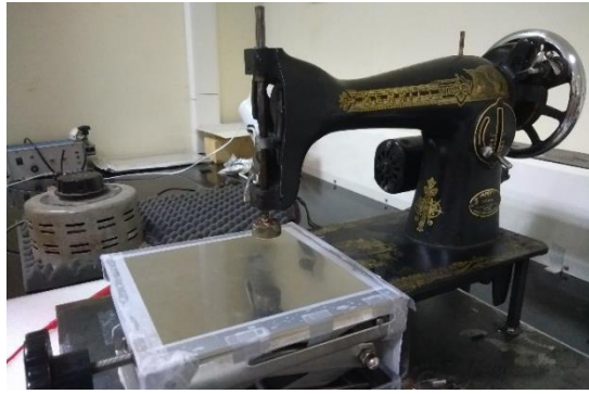
Figure 6-8 Impact test setup made up of a modified sewing machine connected to a potentiometer.
