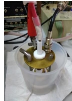
Figure 5-13 Upper view of the sample holder submerged in dielectric fluid (FC40).
