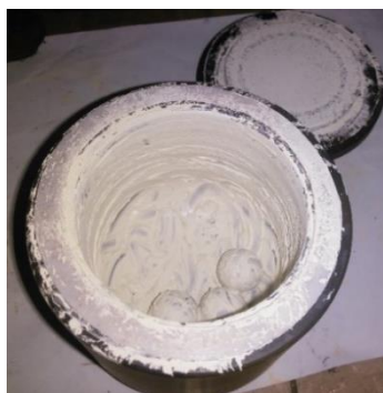
Figure 3-17 Drying LP PZT mixture overnight at T_R after second ball milling.
