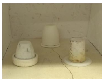
Figure 3-11 Sealed HP PZT pressed compositions placed inside a Lenton Furnace before calcination.
