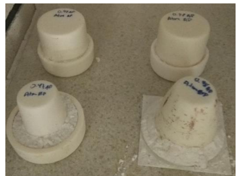
Figure 3-24 Sealed alumina crucibles inside the Elite Chamber Furnace before sintering.
