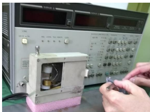
Figure 5-22 Data acquisition system used to calculate the figures of merit of the poled PZT disks.
