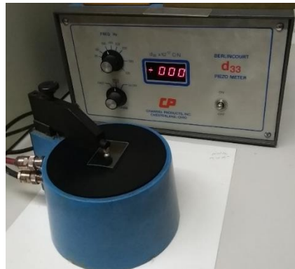
Figure 5-19 Berlincourt meter used to measure the piezoelectric charge coefficient ( d_{33} ) at 100Hz.
