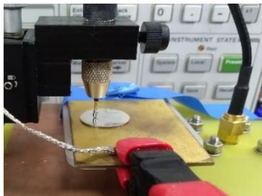
Figure 6-1 Impedance analyser (4395A) setup used to obtain the impedance of the PZT samples.
