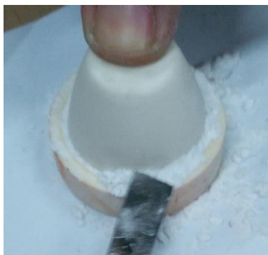
Figure 3-23 Alumina crucible being sealed with alumina powder before calcination at 800°C.
