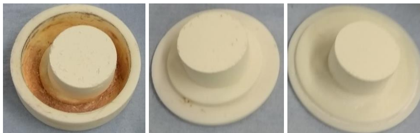
Figure 3-15 Resulting pressed pellets of high purity PZT compositions 0.46 (left), 0.47 (centre) and 0.48 after calcination at 800°C.
