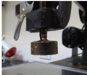
Figure 6-9 Weight of 40N used during the controlled impact tests for the PZT samples.
