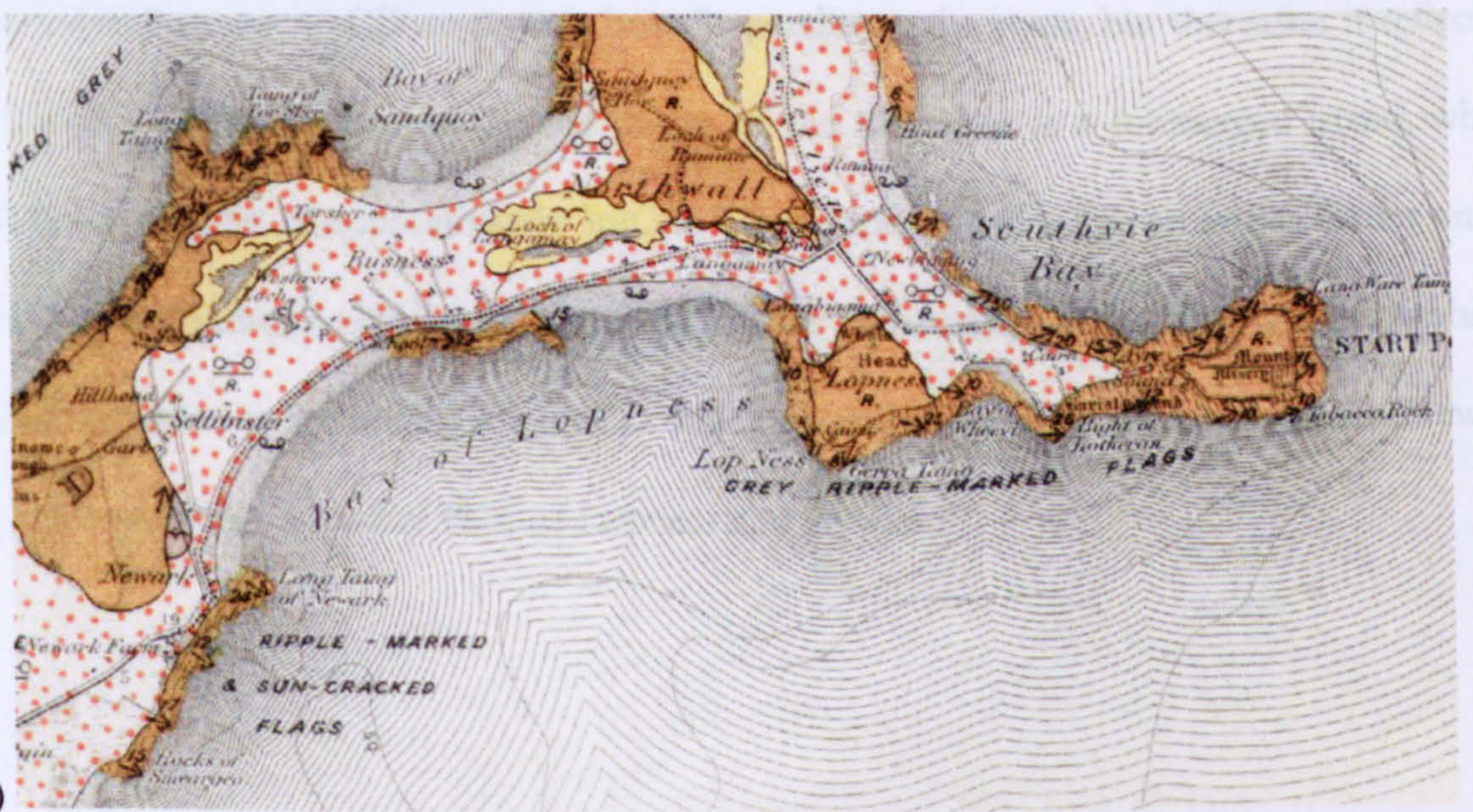
Figure 4.3 (A) Bathymetry (Admiralty chart 2250) and the (B) Geology (BGS sheet XX) of the Bay of Lopness Note geology is shaded with Rousay Flags (brown), windblown deposits (speckled) and alluvium (yellow).
