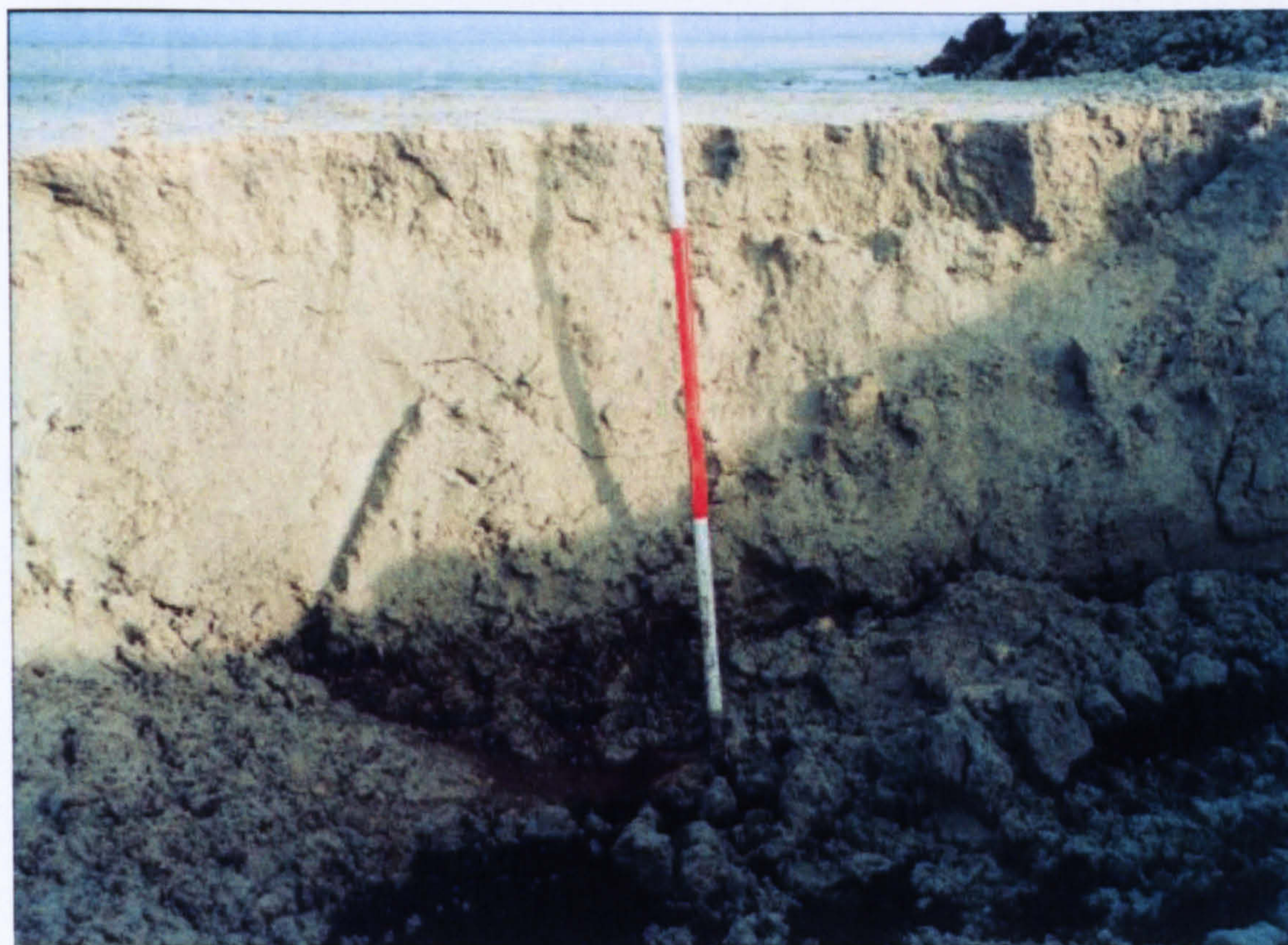
Figure 4.32 Photo of profile shown in Figure 4.31. Note the sand layer lies above a shell layer, below which the peat and till is visible. The peat is spatially limited - present in the foreground but not towards the wall of the pit.
