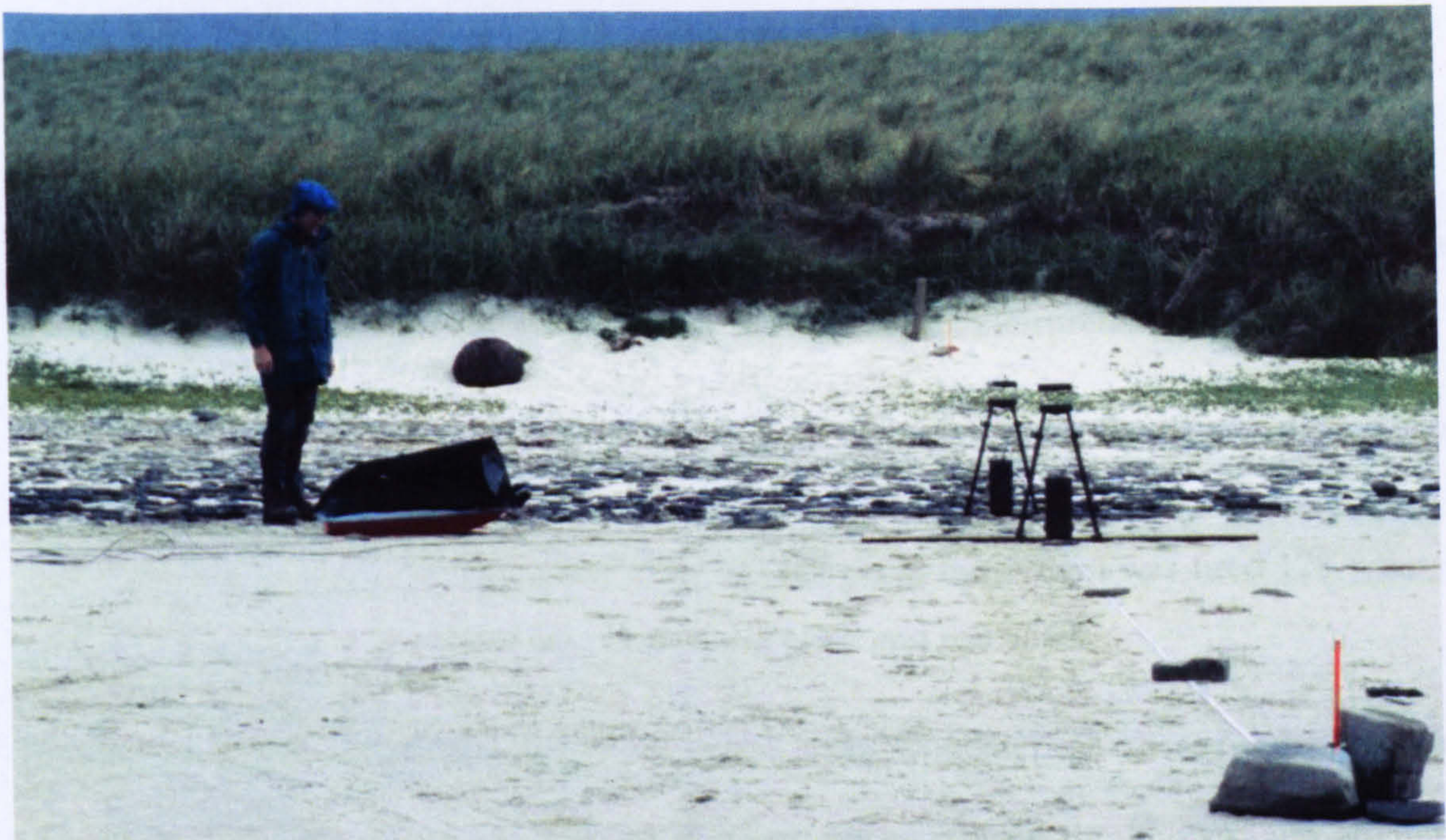
Figure 3.12 The PulseEkko 100 system being tested in the dunes and sandflat of Cata Sand. Note the sledge contains the laptop, console and battery, and has been pulled closer to the antennas for the purpose of the photograph. Also during these early tests a cloth tape-measure was used, later surveys used a set length of string to measure step size.
