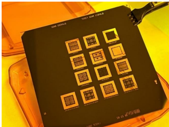
Figure 5.2 Photograph of photolithography mask used for the fabrication of \text{MoTe}_2 FETs as fabricated by the external company.
