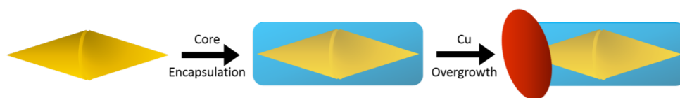
Figure 1.10: Schematic of the synthesis of asymmetric Au (yellow)/Ag (blue)/Cu (red) nanostructures, adapted from 69 .
