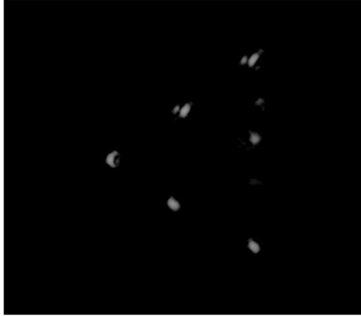
Figure 4.15: Images extracted from the original video showcasing the MPLC’s operation. Some spots are sharp (a, c, f), while others are less so; this is due to imperfect alignment of the optical setup.
