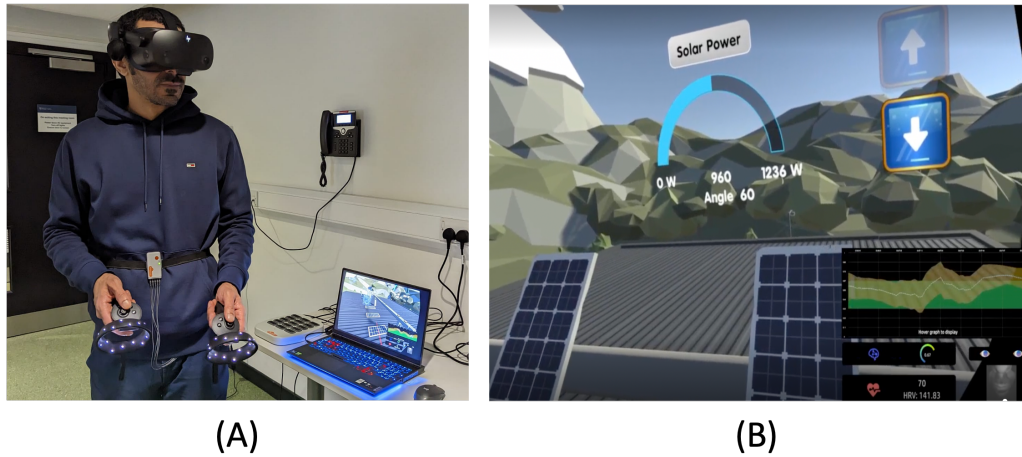
Figure 4.8: The experiment setup. (A) the user is wearing the ECG sensor and the HP headset to perform the VR application. At the same time, the application was live-streaming and recorded on a laptop. The picture was taken from a VR lab at the University of Glasgow. (B) The screen of the OBS studio where the overlay app transparently appeared for casting the heart rate and cognitive load data from the HP headset.
