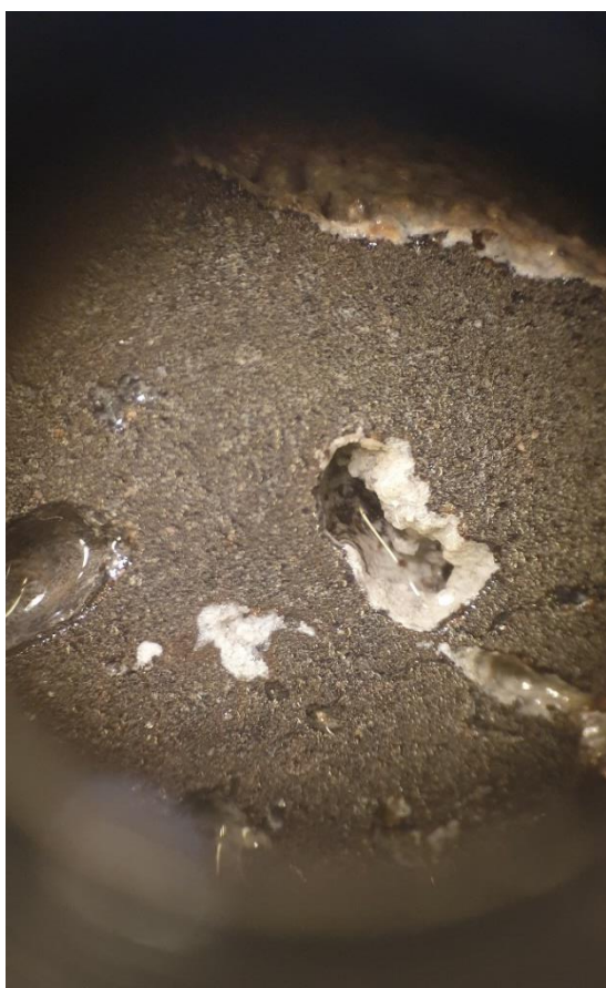
Figure 6.4: A view of one of my slag samples through an optical microscope, during sample preparation for the SEM. White deposits of calcite can be seen precipitated into pore spaces (photograph courtesy of Connor Brolly).
