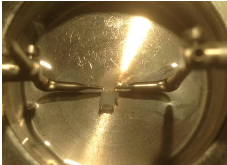
Figure 2-4 Representative picture of a rat aortic ring mounted in the small artery wire myograph.
