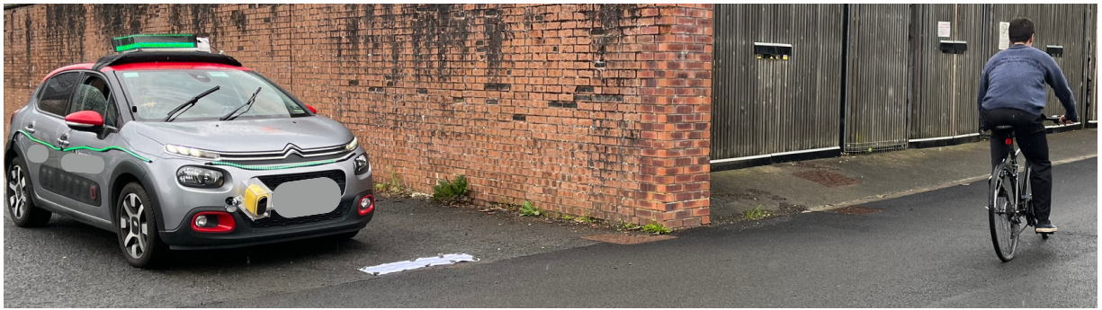
Figure 4.22: Photograph from a pilot study comparing the visibility of LED lights and road projections. Road projections were barely visible in sunny conditions.
