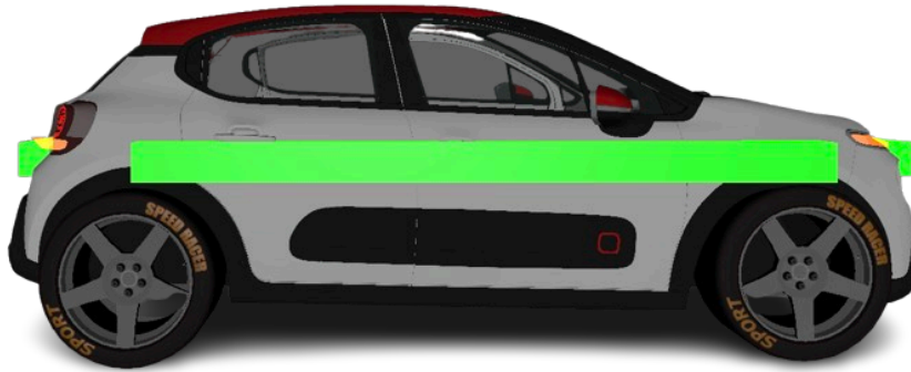
Figure 7.1: The LightRing eHMI: LED strips around the AV that use colour-coded red/green signals to communicate AV intentions (not-yielding/yielding). LightRing is green in this figure, meaning the AV is yielding.
