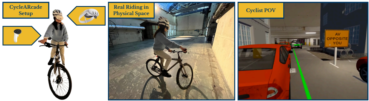
Figure 5.10: The study hardware and setup. The left photograph shows a participant instrumented with a mixed-reality headset and a controller to simulate a smartwatch. The middle photo shows a participant riding in real physical space while wearing the headset. The right photo shows the participant’s POV in the headset.
