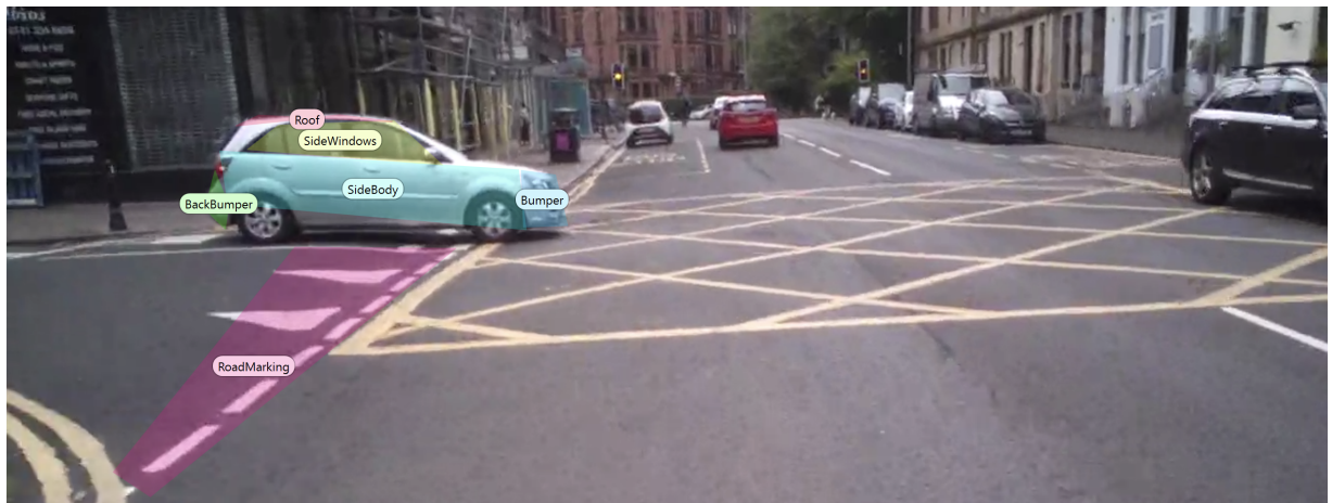
Figure 3.9: A screenshot from the Tobii Pro Lab AOI tool; AOI shapes are placed on relevant areas, and dragged accordingly frame-by-frame.
