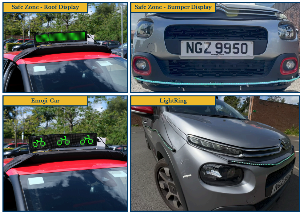
Figure 4.21: Real prototypes of the eHMIs. These were built using LED strips and an LED matrix. The top row shows photographs of Safe Zone. The left photo on the bottom shows Emoji-Car, and the right photo shows LightRing.
