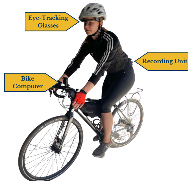
Figure 3.7: An instrumented cyclist. They were given Tobii Pro Glasses 2 eye-tracking glasses, which also featured a recording unit connected via cable. Cyclists also had a bike computer to log their commutes.
