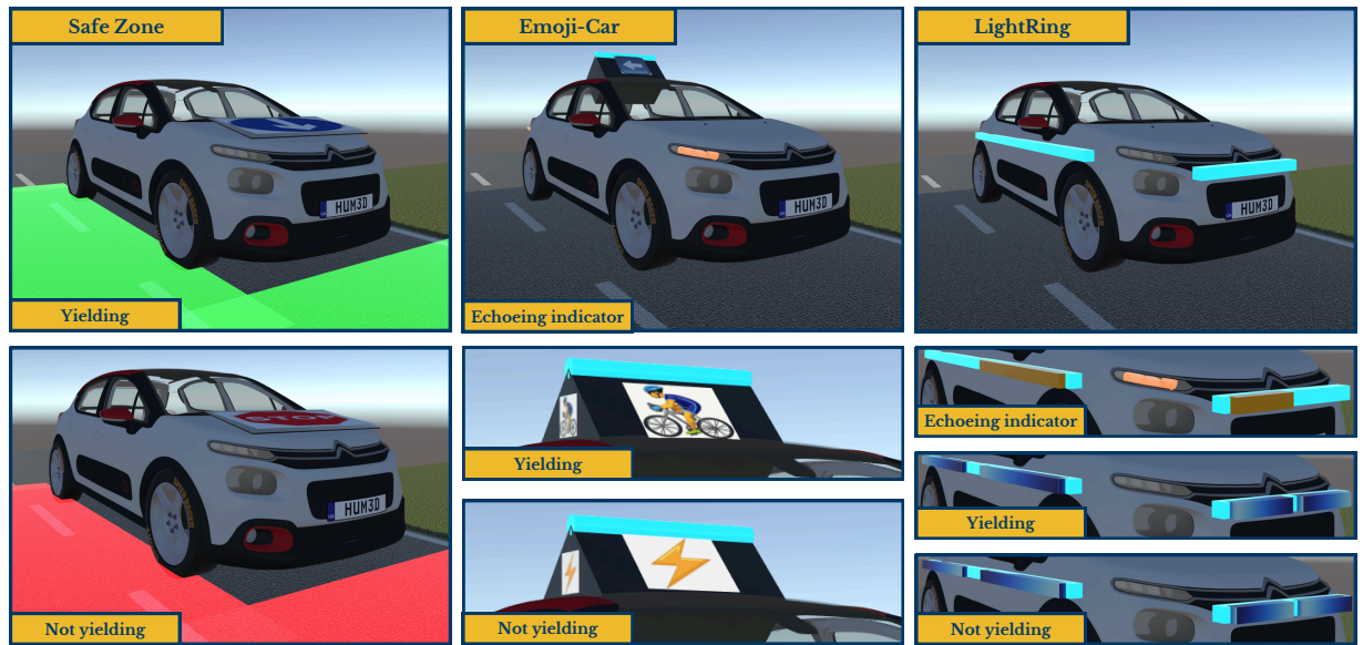
Figure 4.9: The evaluated eHMIs as implemented in VirtuRide. The photos on the left show Safe Zone; the middle show Emoji-Car; the right show LightRing.
