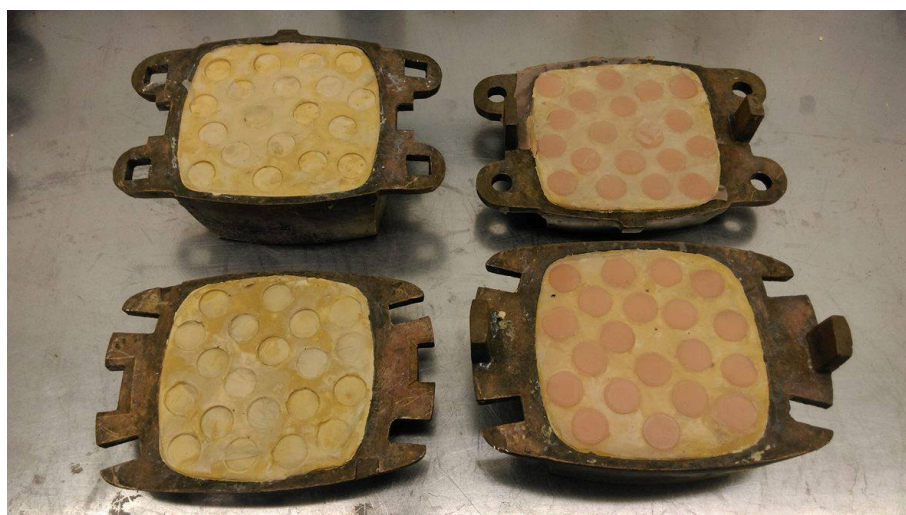
Figure 4.1: Example of the bespoke flasks used to fabricate discs of denture base materials.
