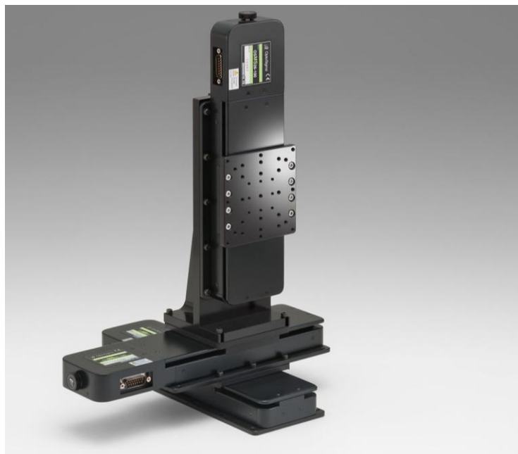
Figure 4-9 Optosigma's 3 axis motorised stage that was used in this work.
