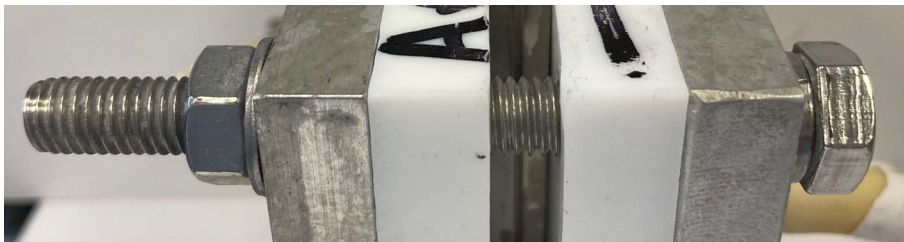
Figure 7: Placing washers on eight M8 (8 mm × 75 mm) hex bolts (fully threaded setscrew) and put them in position around the cell. At the end of each bolt, place another washer and a nut. Ensure that the torque wrench is set to 5.65 Nm and attach the size 13 fitting. Use a spanner and torque wrench to tighten each bolt. The wrench will click when each bolt is torque-tightened to 5.65 Nm.
