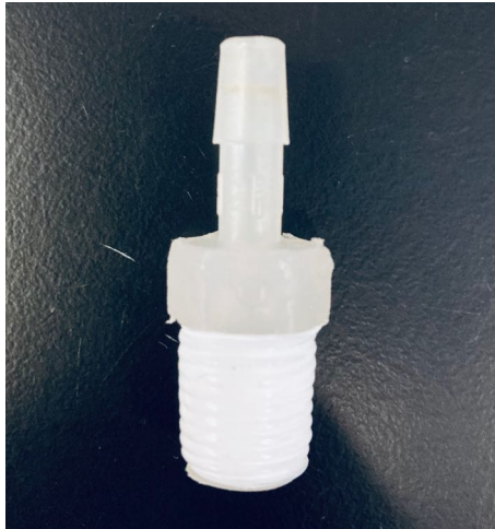
Figure 4: Wrapping PTFE tape on four polypropylene hose barbs/fittings (Masterflex fitting, polypropylene, straight, hose barb to threads; size: 6.35 mm inner diameter \times 6.35 mm national pipe thread (NPT) (M)).
