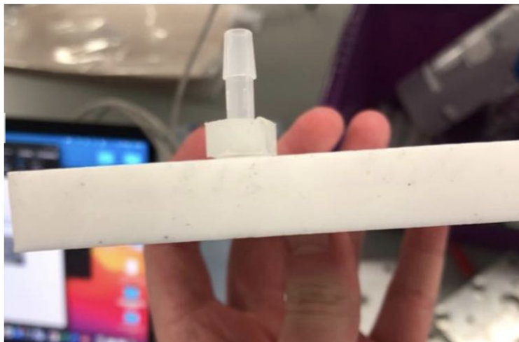
Figure 5: Attaching the four tube fittings into four PTFE insulating plate.
