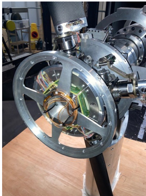
Figure 3.13: Telemetry carrier mounted on the rotor hub attached to power and signal cables that run through the propeller shaft from the inductive coil system.
