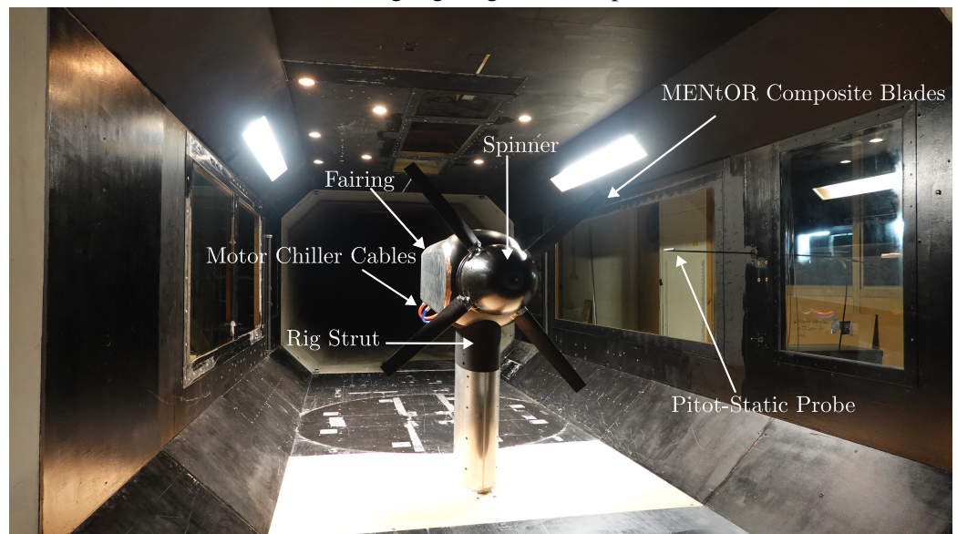
(b) UKNRR installed in the De Havilland wind tunnel.
