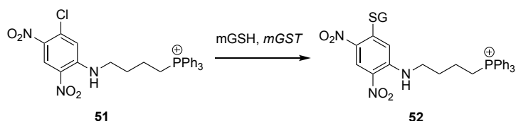
Scheme 18. mGST-catalysed S_NAr reaction of MitoCDNB 51 and mGSH.
