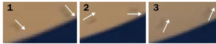
Figure 37. The magnetic nanoparticles under micro-scope and the rotation under 1Hz field from coil in one period.
