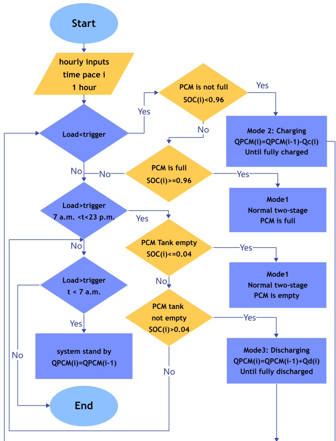
Figure 4.7 Flowchart of the simulation for a flexible two-stage heat pump: Cooling application.
