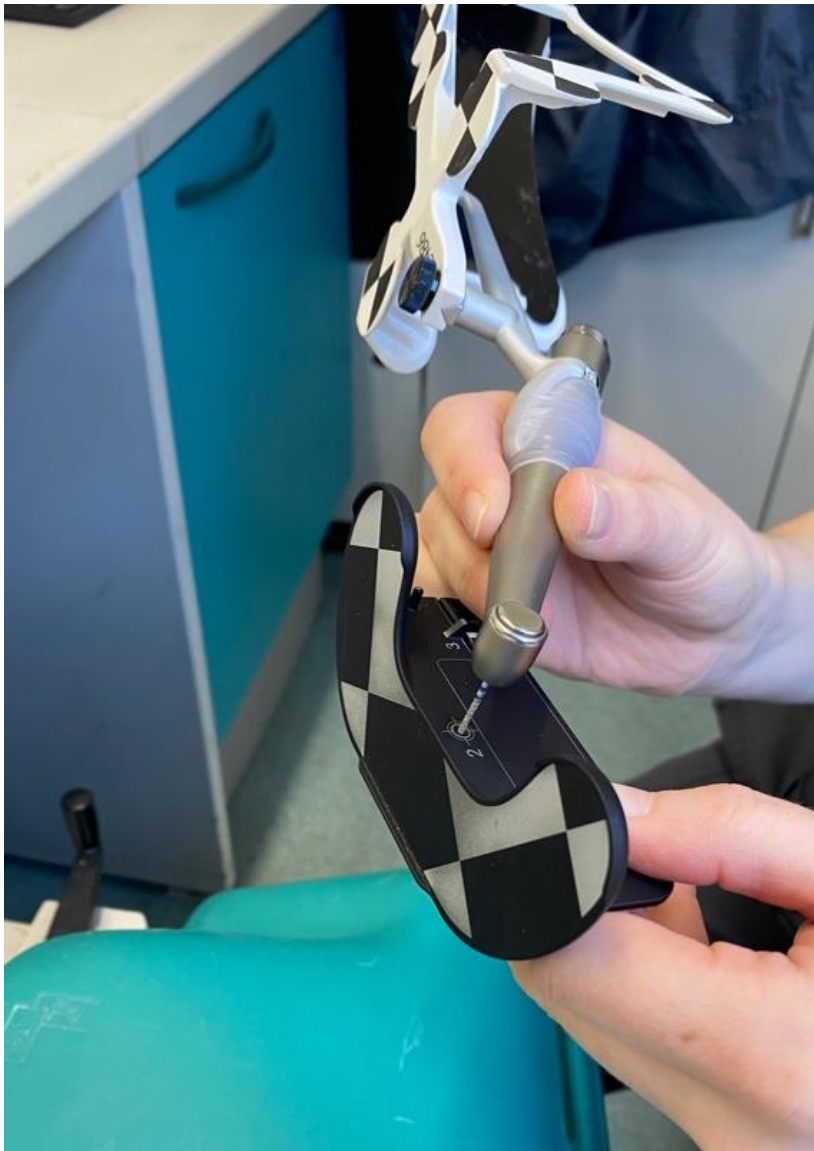
Figure 5-16 - Drill-tip calibration. Demonstrates the bur secured in the handpiece with the tip of the bur placed onto the Calibrator tool dimple to calibrate the drill tip.
