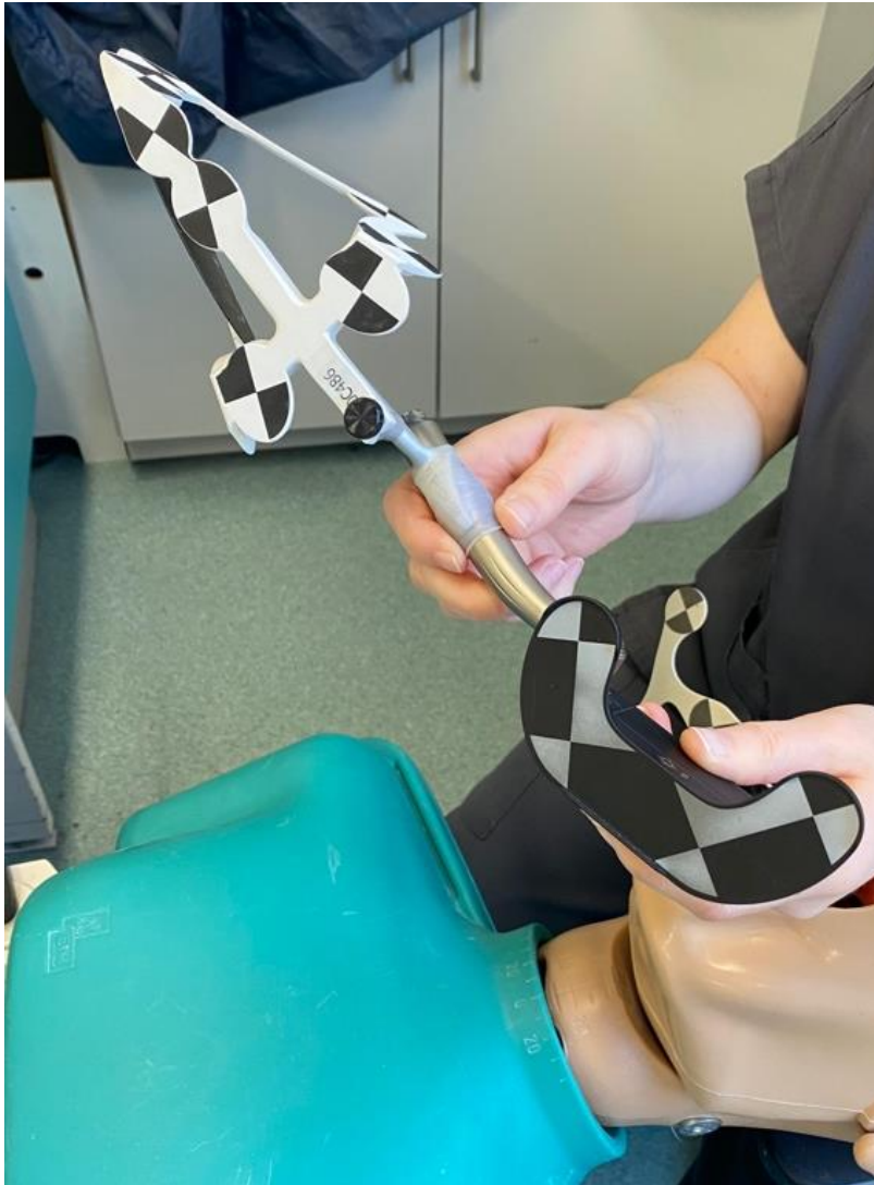
Figure 5-15 - Axis calibration. Demonstrates the DrillTag secured to the handpiece (held with right hand) and the Calibrator tool used to calibrate the drill axis.
