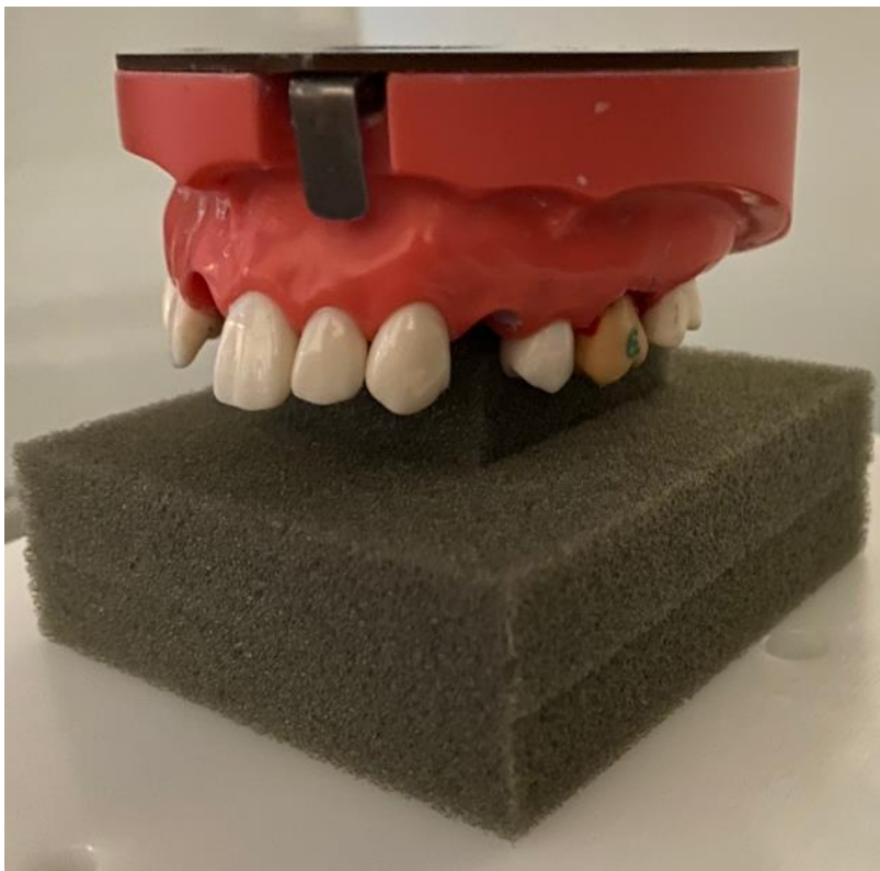
Figure 5-6 - CBCT set-up with the 3D-printed tooth mounted in the Nissin jaw model. Demonstrates anatomic and raised positioning of jaw model to prevent any tooth displacement between use of the jig and the CBCT. The CBCT facilitated planning on the Navident software.
