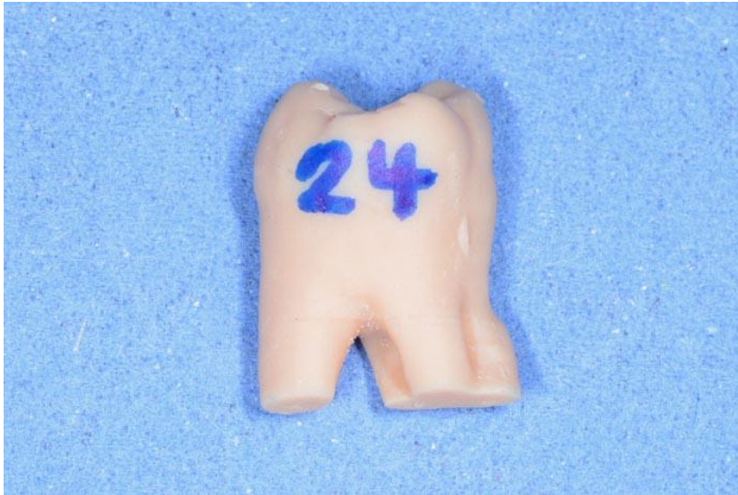
Figure 5-2 - Photograph showing a sample of the selected 3D-printed tooth for the study. Demonstrates the perpendicular root section which allowed drainage of resin following 3D printing.
