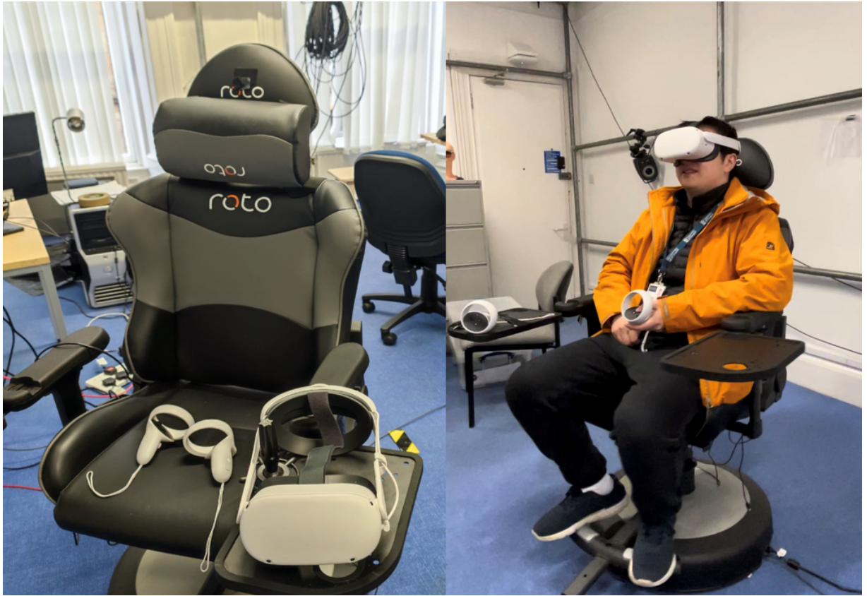
Figure 3.2: On the left is the RotoVR rotating chair. On the right is a participant undergoing rotational motions on the chair.
