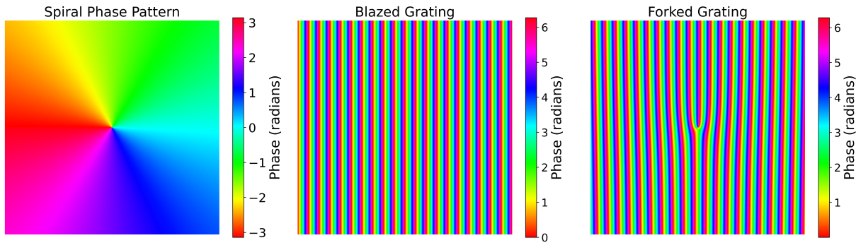
Figure 4.9: Example of the combination of a spiral phase pattern and a blazed diffraction grating, which can be combined to give a forked diffraction grating. When displayed on the SLM, the incoming light is diffracted, turning the imaging configuration from on-axis to off-axis and allowing for better modulation of the incoming light.
