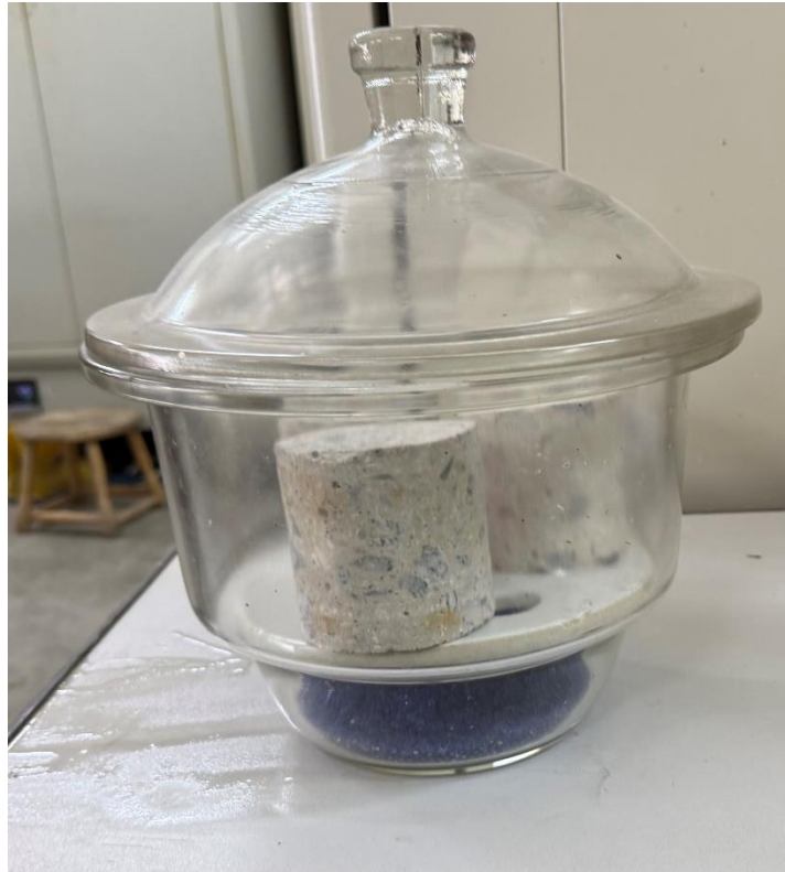
Figure 3.11: Desiccator used for storage before water absorption test
