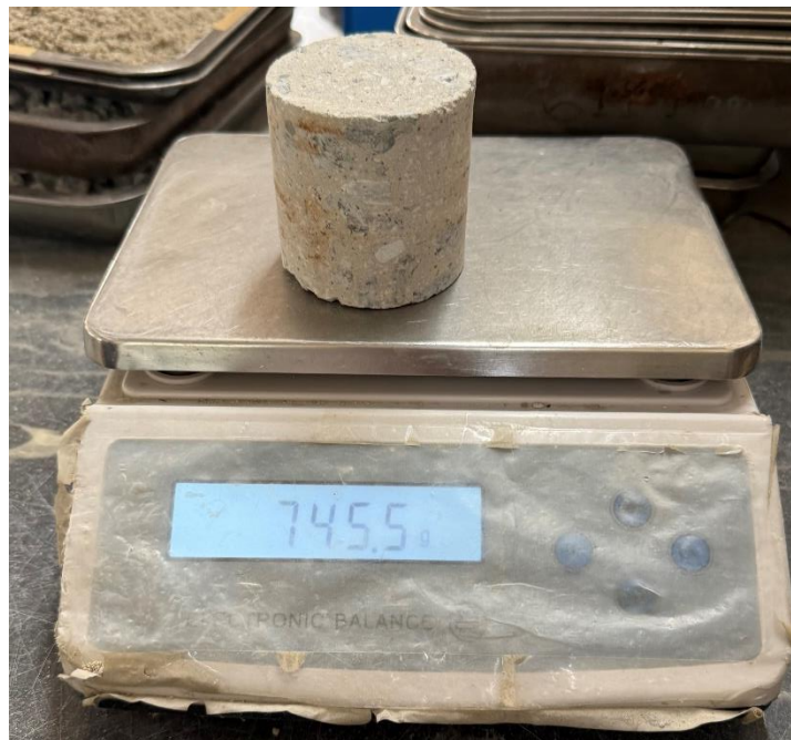
Figure 3.12: Water absorption specimen weighs in before submerging in water
