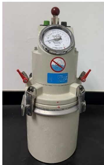
Figure 3.1: Air Entrainment Meter for the measurement of Air Pore Content
