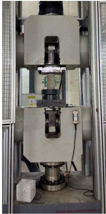
Figure 3.4: Shenzhen Wance Testing Machine DTC 500 UTM
