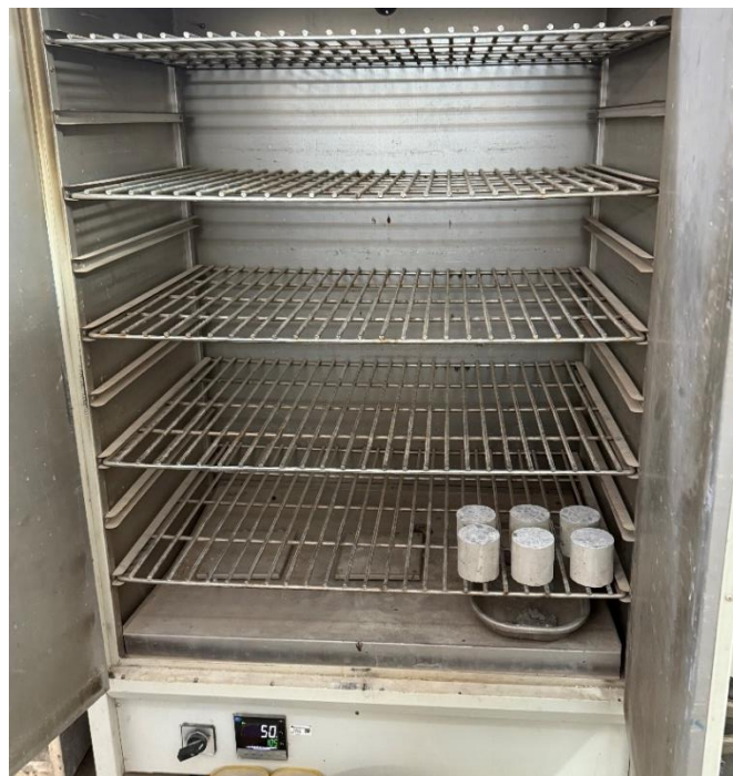
Figure 3.10: Oven used for water absorption specimen prior to testing
