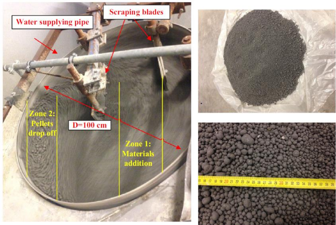
Figure 2.3: Process of artificial aggregates produced using cold-bonded pelletisation technique in concrete applications (Tang & Brouwers, 2018)
