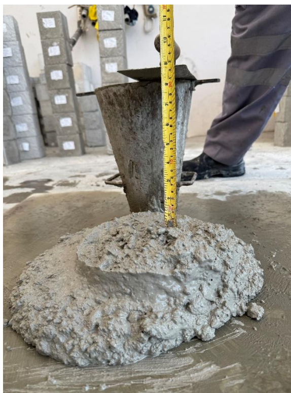
Figure A.10: P0 Slump Photo
