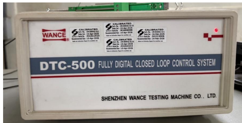
Figure 3.5: Data logger for UTM
