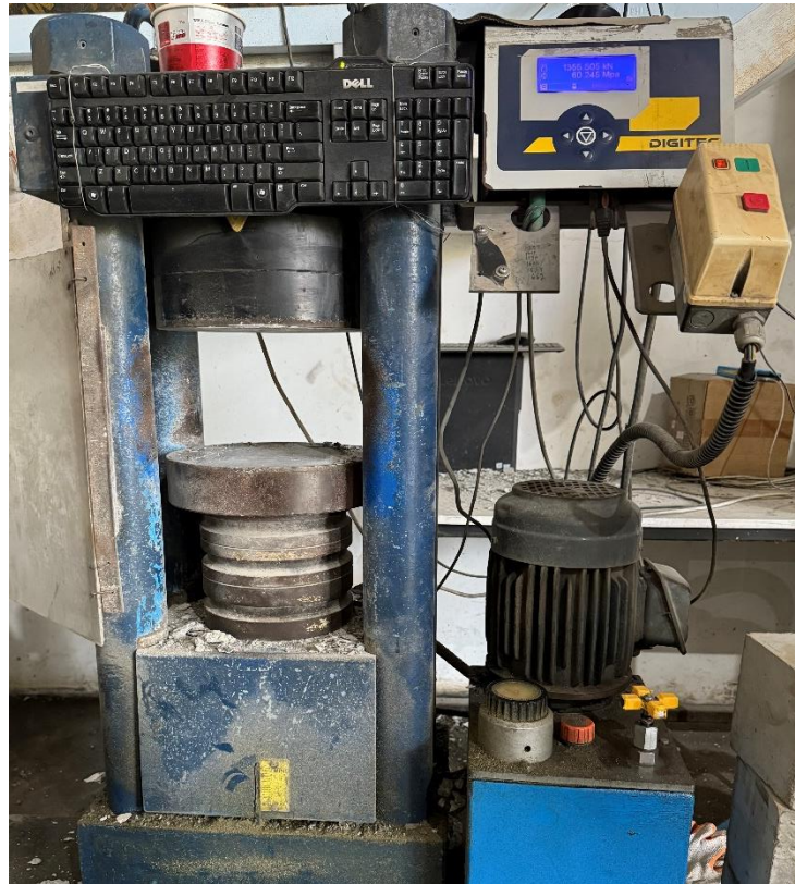
Figure 3.3: Matest concrete compressive test machine 2000 kN
