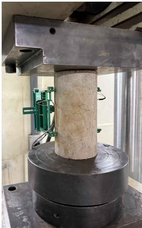
Figure 3.7: Testing setup for MOE
