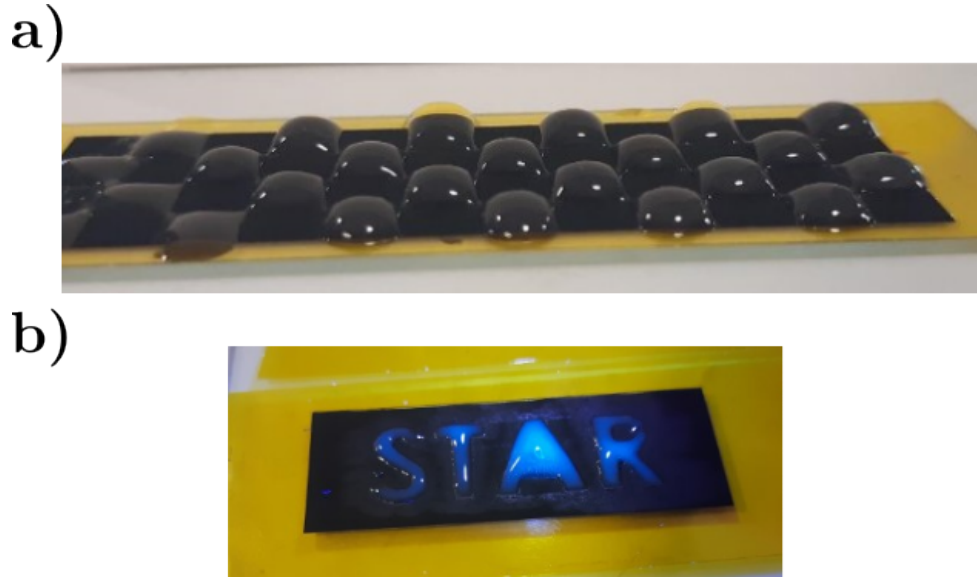
Figure 6.5: a) Chequerboard pattern on PI film demonstrating combined hydrophilic and hydrophobic regions; b) Tonic water illuminated under UV light, highlighting the controlled liquid containment within the patterned areas.
