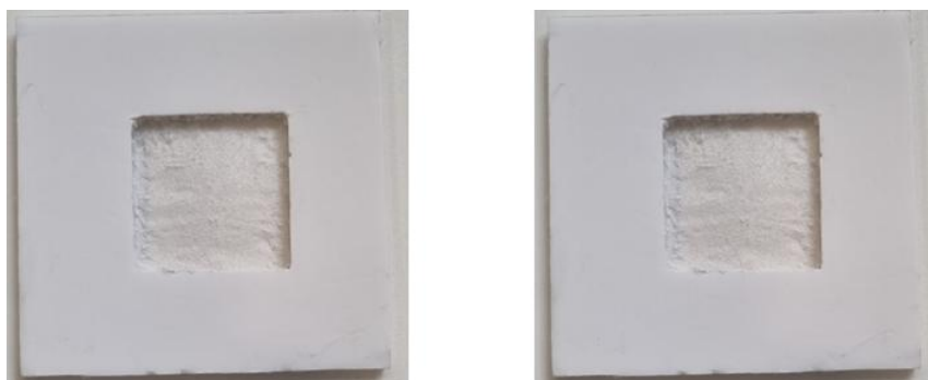
Figure 3.1. Foamboard structure used to support the Ti felt electrode during the air-spraying of the \text{IrO}_2 catalyst onto the Ti felt.
