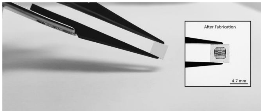
Figure 2.2.1 Single-crystal CVD diamond substrates before and after fabrication [2.19].
