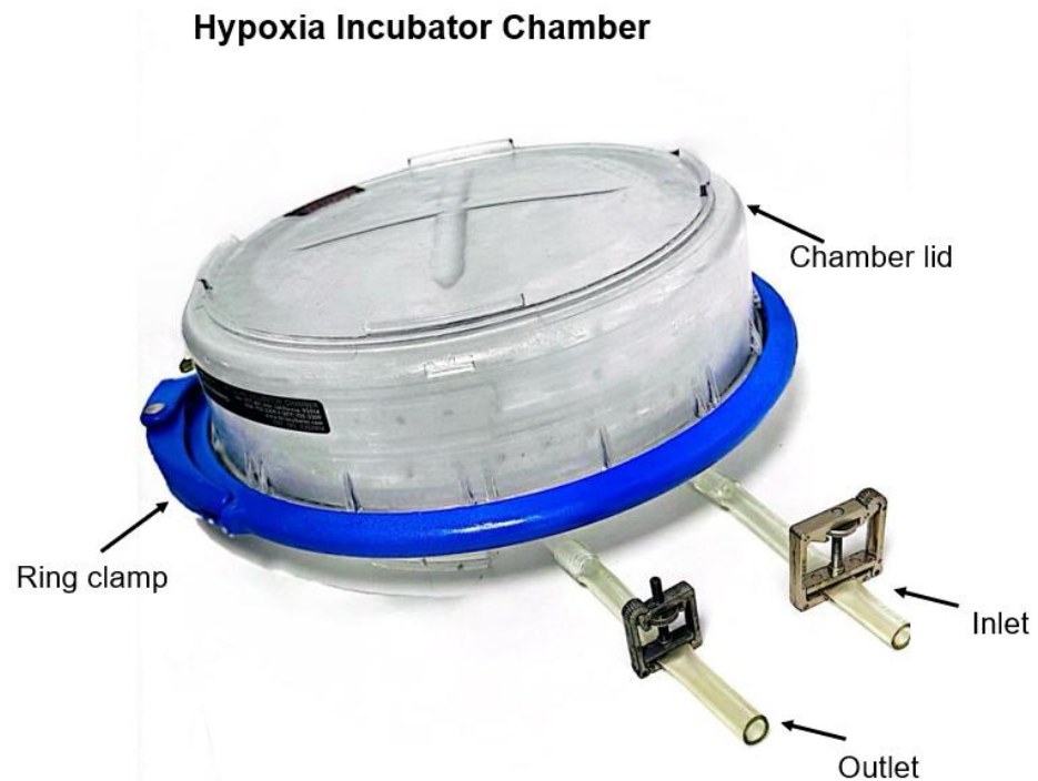
Figure 2-5 Modular incubator chamber for hypoxia induction.
