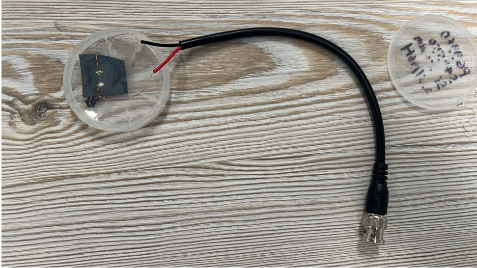
Figure 4.19: A successfully fabricated Tai-Chi PCA has been connected to BNC cable for applying bias voltage.
