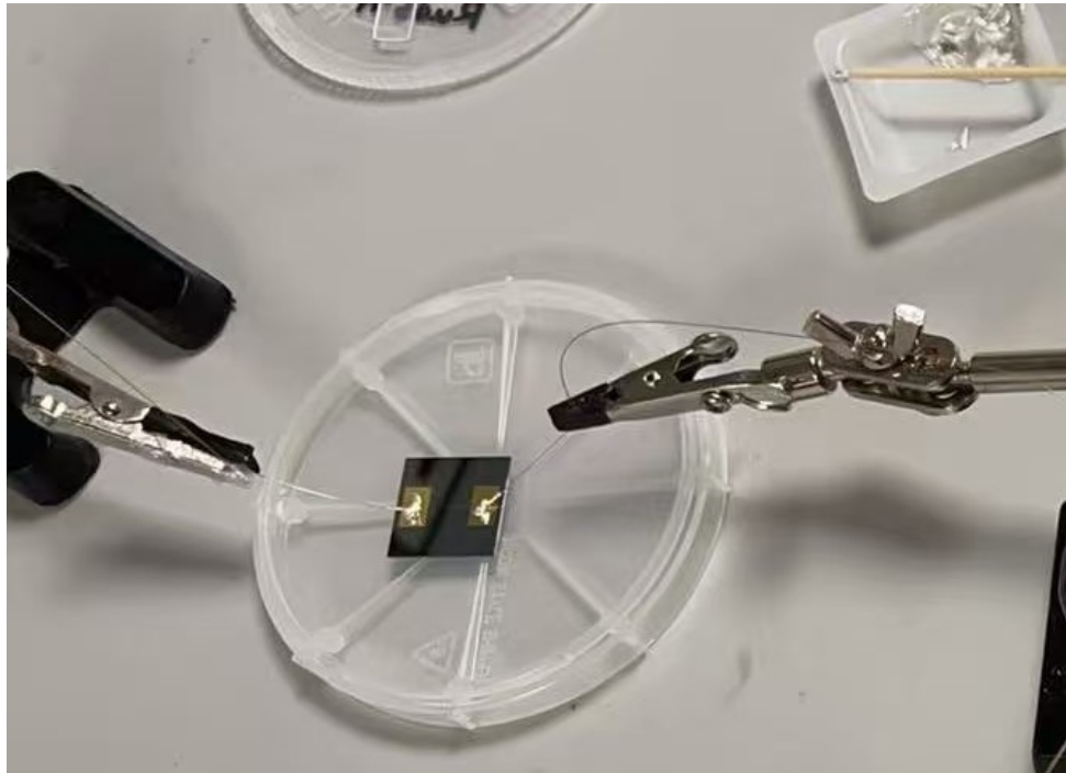
Figure 4.18: Connecting wires to the biasing pads of Tai-Chi PCA using silver conductive gel.
