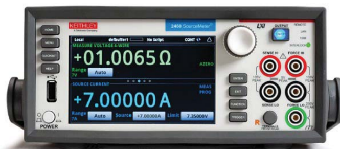
Figure 3.20: A picture of the Keithley-2450 source measurement unit. The surface current of the fabricated GQD-based THz spiral PCA is detected by such device.
