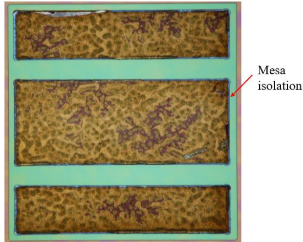
Figure 6.7 Outline of Mesa Isolation profile after Etching Process
