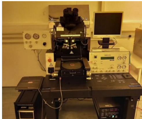
Figure 3. 1 Suss Mask Aligner (MA6) in JWNC for photolithographic patterning
