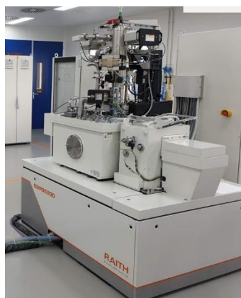
Figure 3. 3 An image of Raith 100 kV EBPG 5200 electron beam lithography tool in the JWNC
