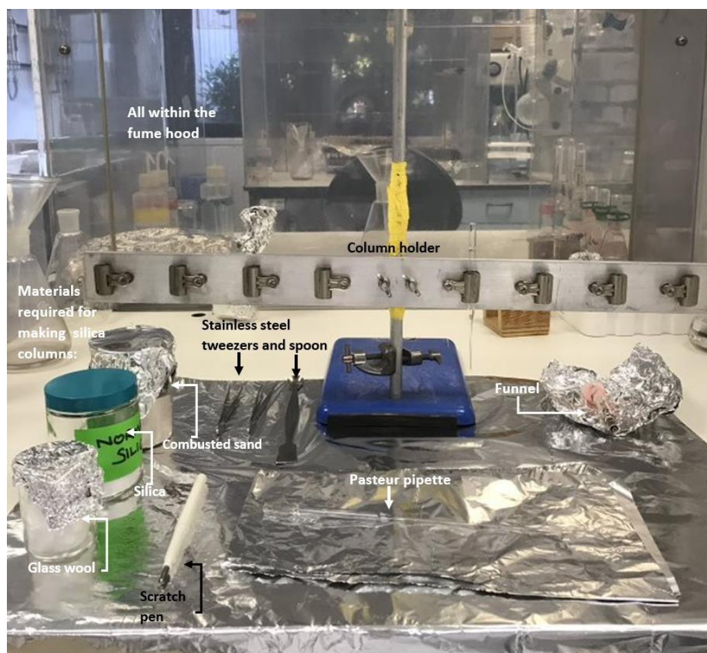
Figure 12- Image depicting labelled equipment and set up required for column chromatography within fume hood
