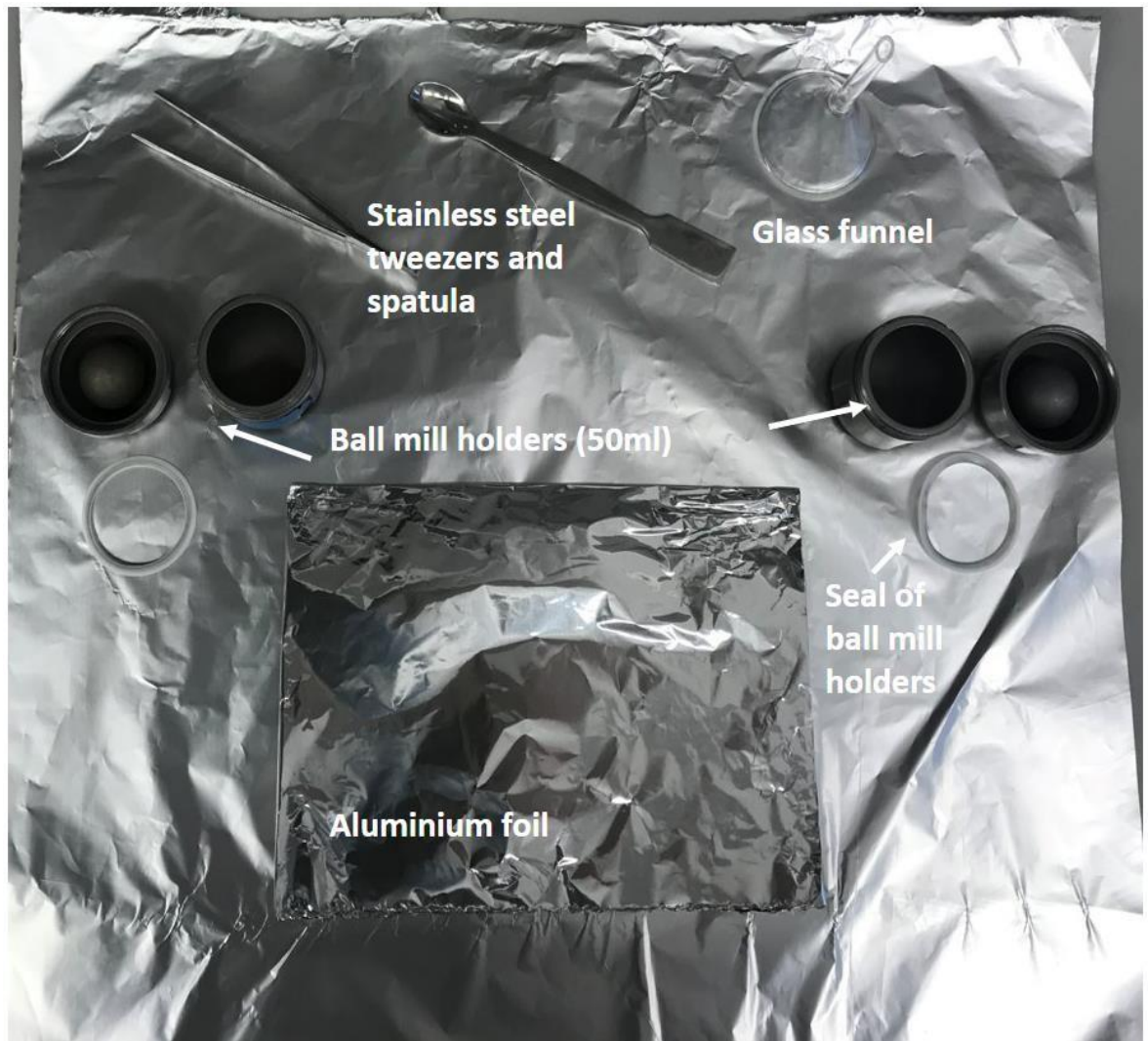
Figure 8 - Image of the set up required for ball mill crushing (ball mill not pictured)
