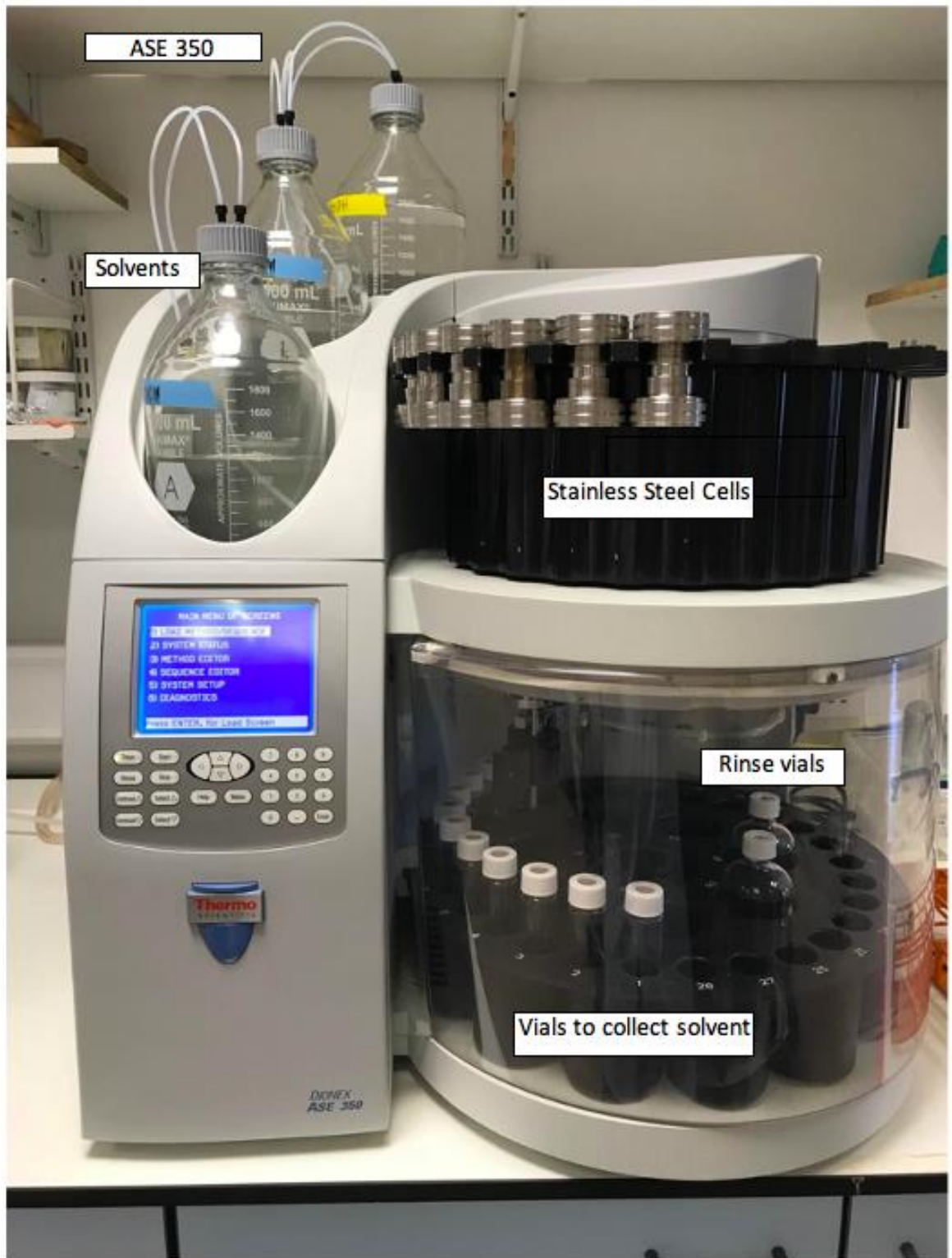
Figure 10 - Dionex 350 Accelerated Solvent Extraction loaded with samples and labelled accordingly within BECS Lab
