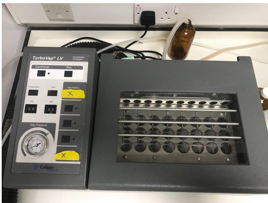
Figure 37 - Techne Sample Concentrator within the laminar flow hood
