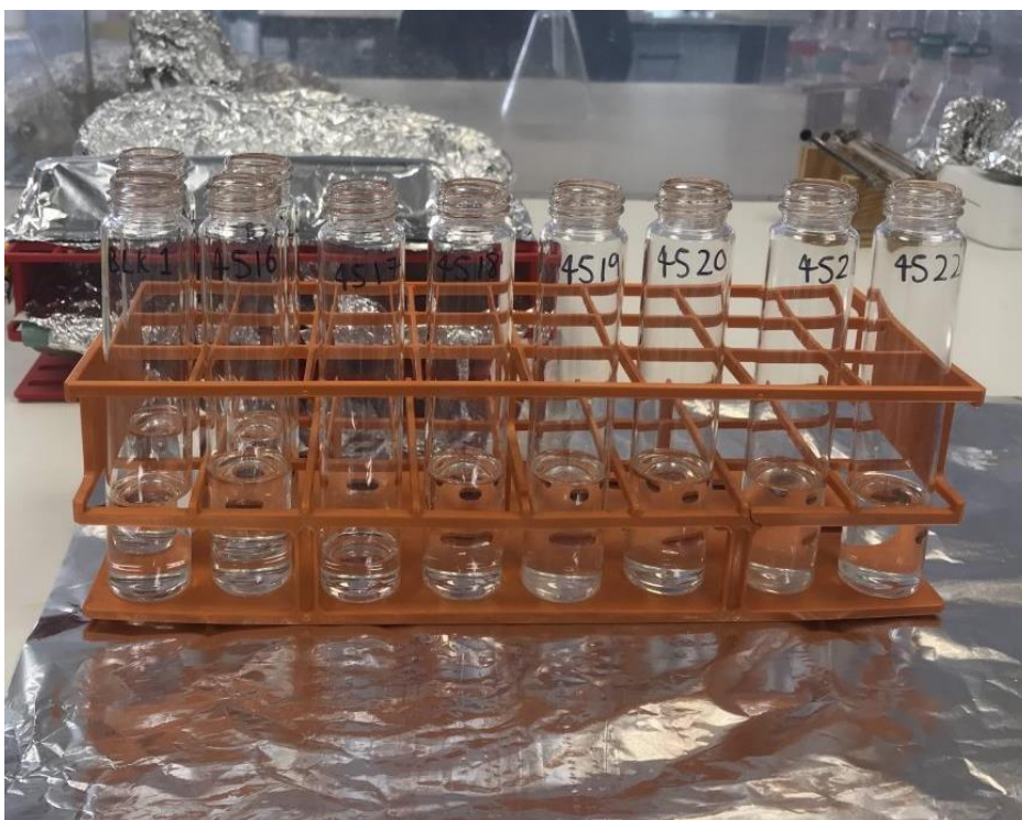
Figure 11- ASE vials labelled with BECS IDs after solvent extraction prior to evaporation stored within the fume hood
