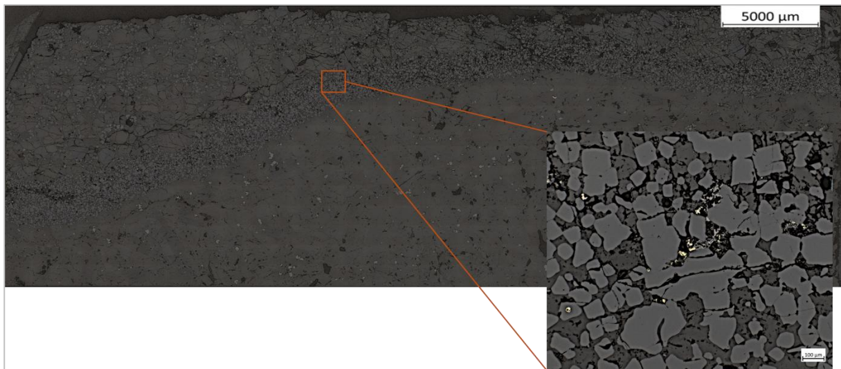
Figure 5.2.2: Optical Stich Image of the chromite seam along the unit 7-8 boundary taken using Zeiss Axio Imager M2M (plane polarised light). Image on the right shows sulphide minerals within the chromite seam.
