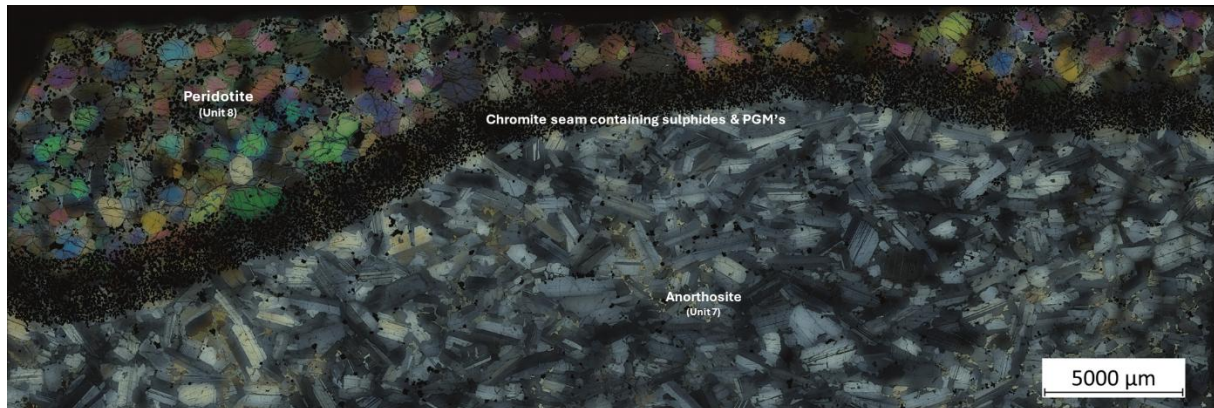
Figure 5.2.1: Optical Stich Image of the chromite seam along the unit 7-8 boundary taken using Zeiss Axio Imager M2M (cross polarised light).
