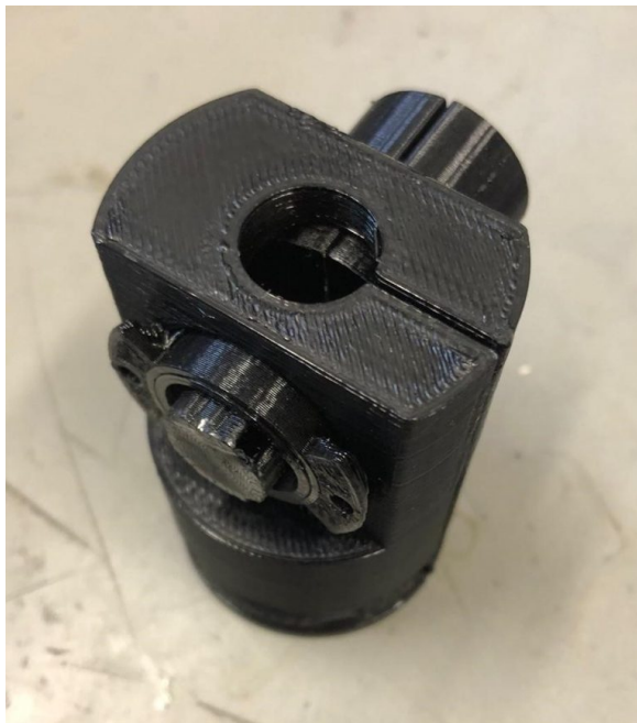
(a) 3D print of the GOSEM LED and QPD subassemblies fitted into a mock-up of the BOSEM main body.
