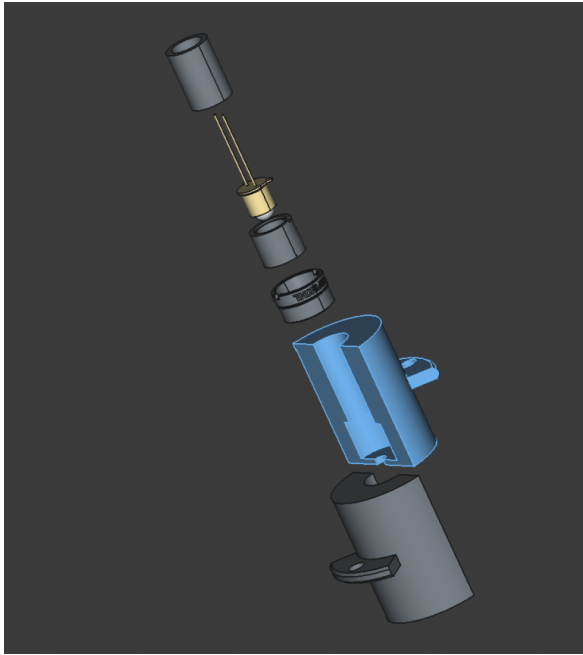
(a) LED subassembly (exploded view). From top to bottom: retainer ring, LED (LED1200L), LED sleeve, an 8 mm-mounted aspheric lens, and the carrier. The carrier is split into two halves to minimise clamping-induced stress on the lens (reducing the risk of fracture) and to simplify integration of alternative lenses, enabling a modular optical package.
