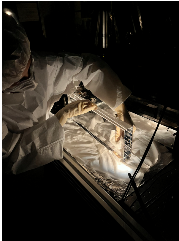
Figure 4.12: Inspection and cleaning of the OMC glass breadboard using high-purity IPA wipes and halogen lighting to remove and detect particulate and fibrous contaminants prior to template bonding.
