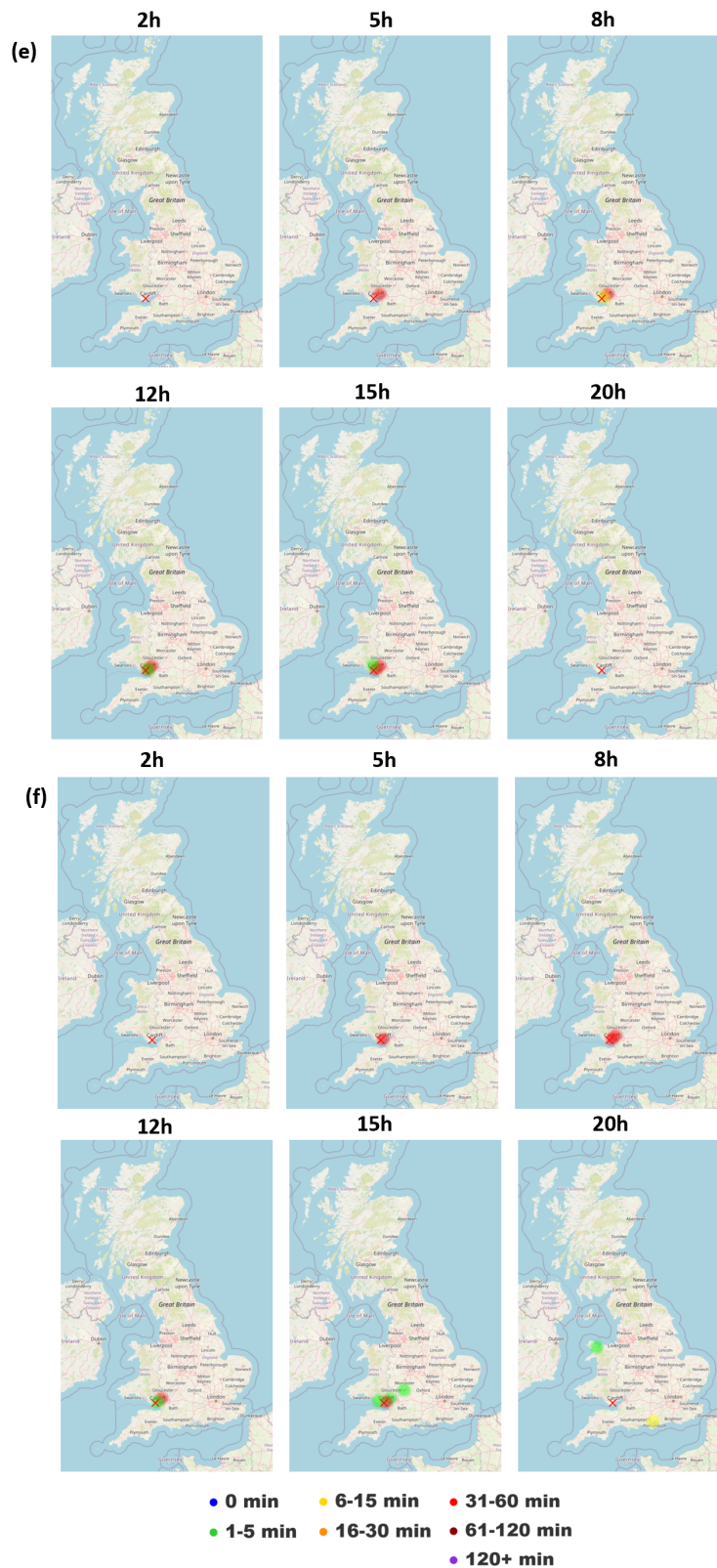
Figure 4.5: Incident View illustrating the impacts caused by an incident in 6 snapshots: (e) and (f) for two incidents from Cardiff due to planned disruptions. Initial incident locations are indicated by a red cross in each figure. From left to right, the figures represent the impacts after 2, 5, 8, 12, 15 and 20 hours after the start of the incident.
