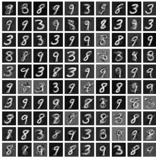
Figure 5.41: Samples generated by LDM. While the overall digit shapes are generally identifiable, many samples exhibit blurriness and structural artifacts, suggesting limitations in the latent representation quality.
