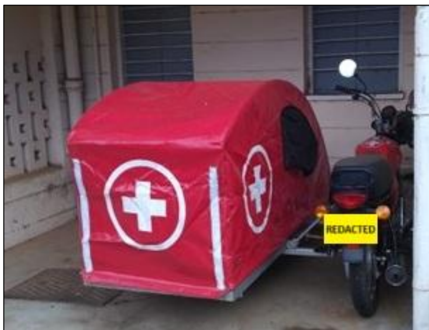
Figure 13: Motorbike ambulance with enclosed sidecar for use in rural SSA. An example of an IHV collaboration resulting in a sustainable solution that addresses health SDGs 3.1 and 3.2.
