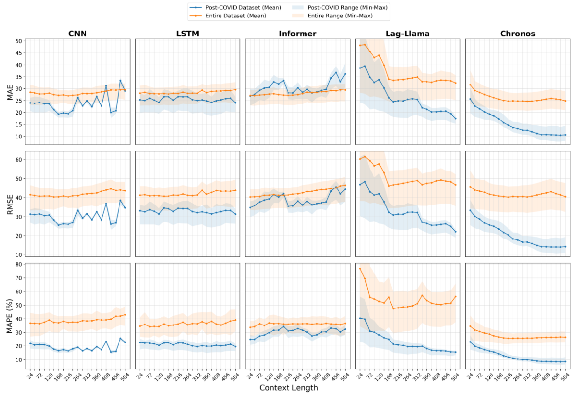
Figure 6-3. Comparison of the post-COVID-19 and entire dataset performance (MAE, RMSE, MAPE) of models across different input lengths.
