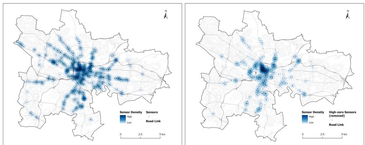
Figure 4-3. Spatial distribution of original traffic sensors (left) and high-zero traffic sensors removed in Step 5 (right) in Glasgow.
