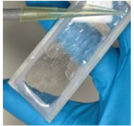
(h) Repeat step (g) on opposite side of mount, confirm both sides fully dried.
