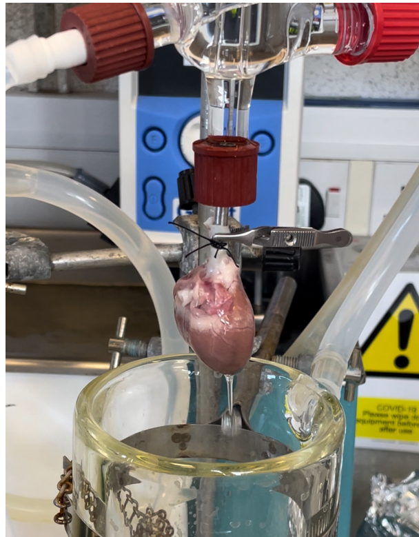
Figure 3.2: Intact rabbit heart cannulated onto Langendorff perfusion assembly.
