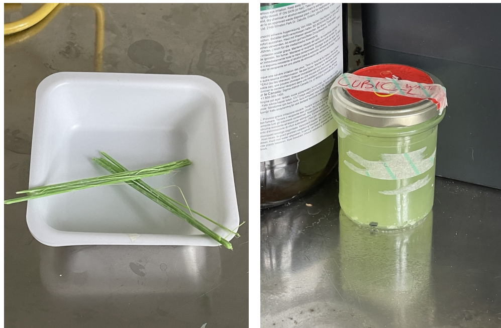
(a) Severely damaged remains of PLA mount after clearing attempt (b) CUBIC-L solution saturated With PLA dye after clearing attempt
