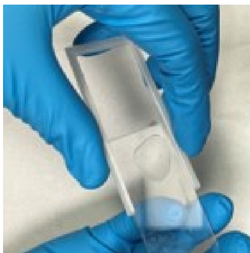
(e) Slide sandwiched sample into mount with internal spacer placed between the slides.
