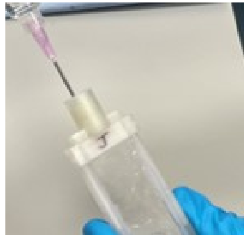
(j) Inject RI Matching Solution slowly via syringe port. Inject till sample immersed.
