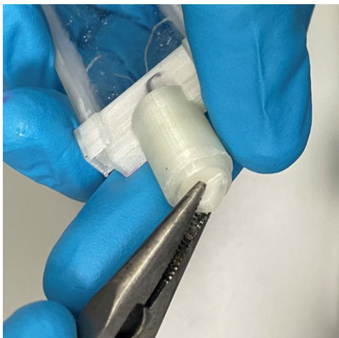
(k) Insert Cap over syringe ports using pliers, ensure fully inserted.
