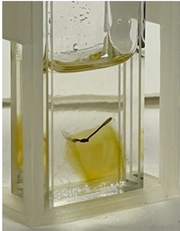
(a) Image of properly orientated spheroid sample in mounted inner cuvette. Excitation light enters inner cuvette from narrow side on the left.
