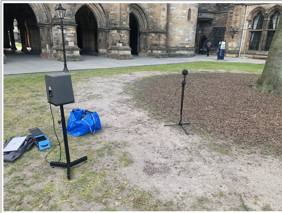
Figure 4.7: Outdoor test environment used for Study 2, illustrating the setup for RIR capture.
