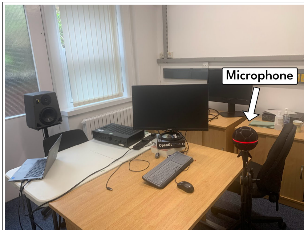
Figure 4.1: Test environment used for Study 1, illustrating the setup for RIR capture. In the user study, the speaker remained in this position and the participant was seated at the microphone position.
