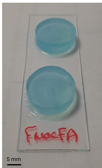
Figure 3.20. FmocFA gels for confocal microscopy. Gels were formed within a 25 mL syringe with the top removed and placed on a glass microscope slide for imaging.
