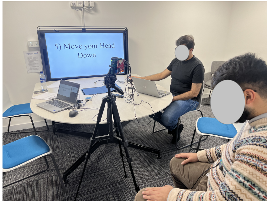
Figure 4.2: Experimental setup for fine-grained motion capture, showing participant seating, mmWave radar placement, and the guidance interface.
