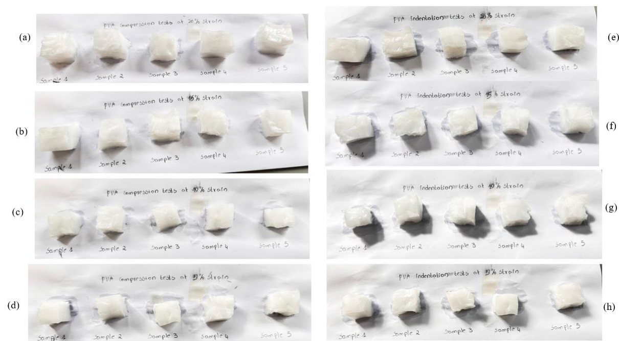
Figure 4.4.1: Compression (a, b, c, and d) and indentation (e, f, g, and h) of PVA hydrogel samples at 20%, 15%, 10%, and 5% strain.
