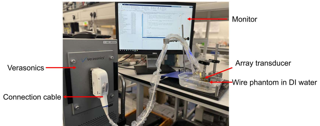
Figure 5.13 Experiment setup for measuring the phantom for resolution measurement.
