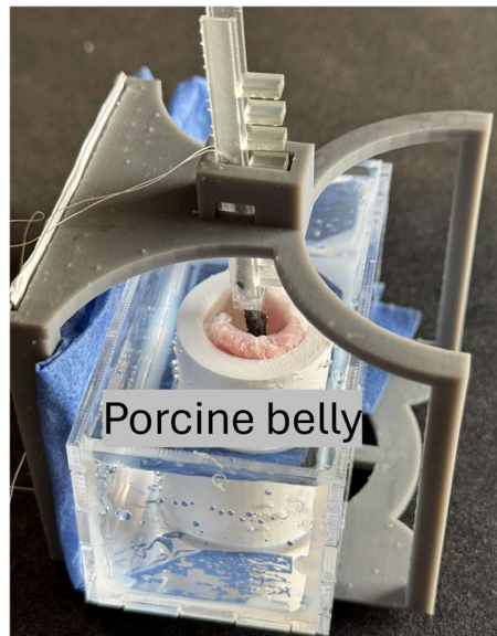
Figure 4.17 Photograph of a section of ex vivo porcine belly mounted for scanning.
