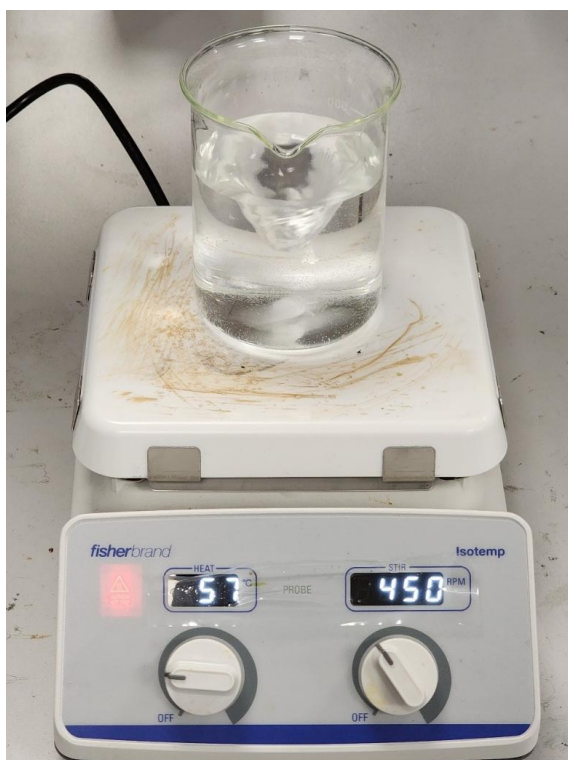
Fig. 3.16: Preparation of a clear, homogenous Ethaline DES at 60 °C with stirring.
