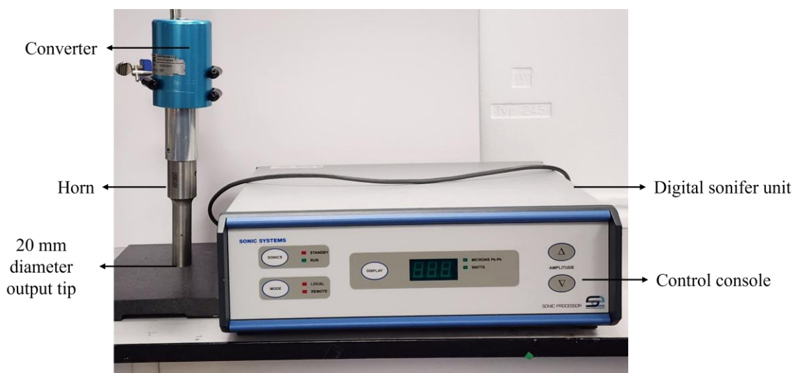
Fig. 3.1: Sonic Systems ultrasonic sonotrode, comprising the sonotrode, the output tip and the control console, to initiate and set input power for a sonication
