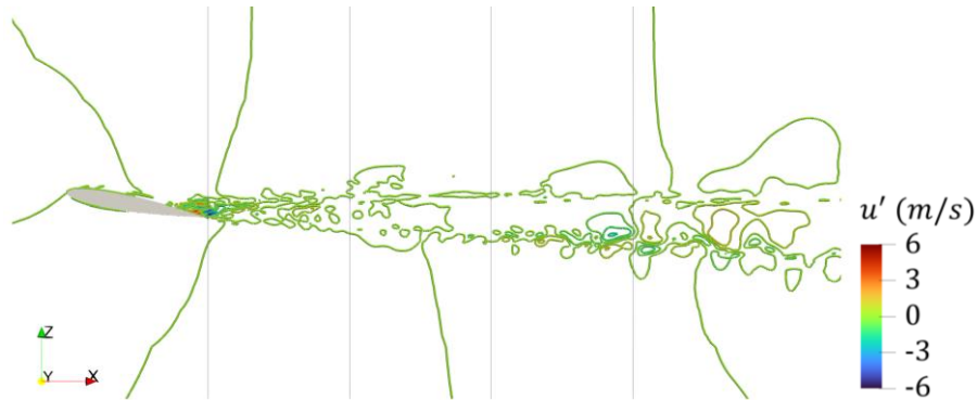
Figure 4.13 Contour in the LES IC domain, coloured by velocity fluctuations u' , view from the wingtip.
