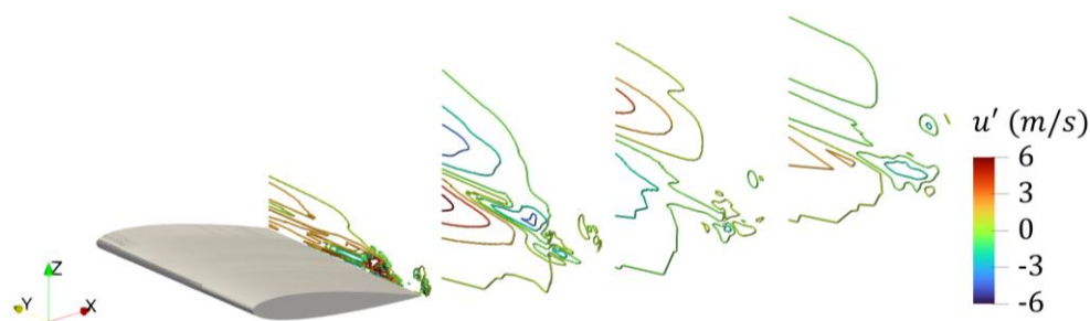
Figure 4.14 Velocity fluctuations contour at planes x/c = 0, 1, 2 , after trailing edge.
